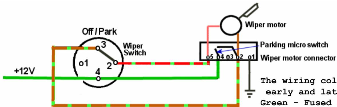
The wiring colours should be common to both early and late motors -
