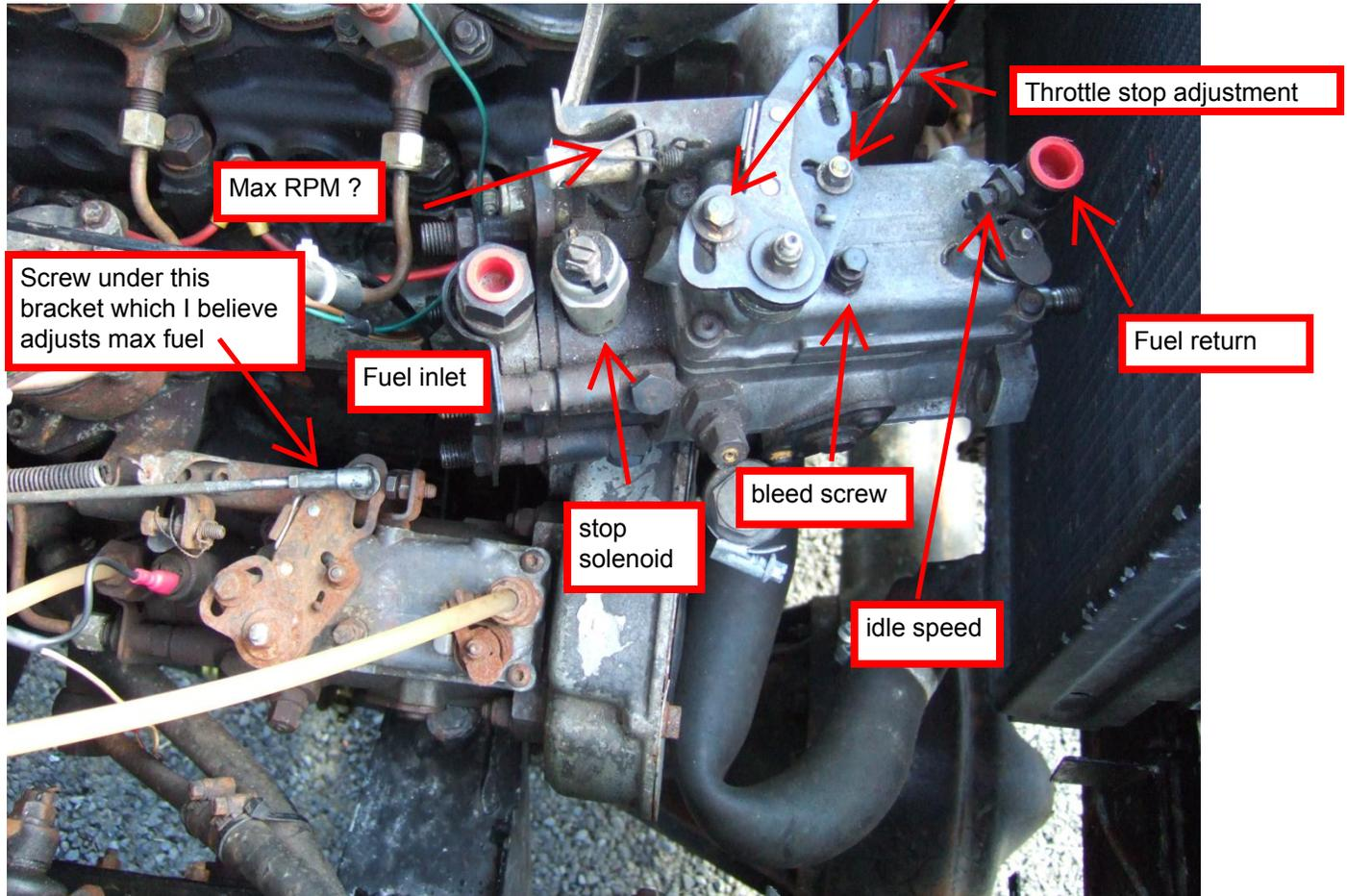
Fitted pump and spare adjusted differently?
