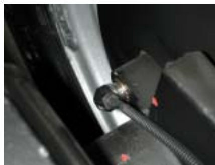
Fig. 15 Installation position of the speed sensor
