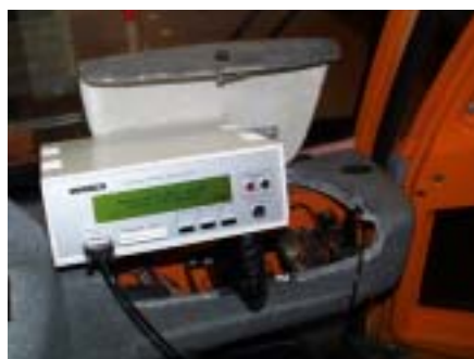
Fig. 21 Diagnostic Controller with connection cable
