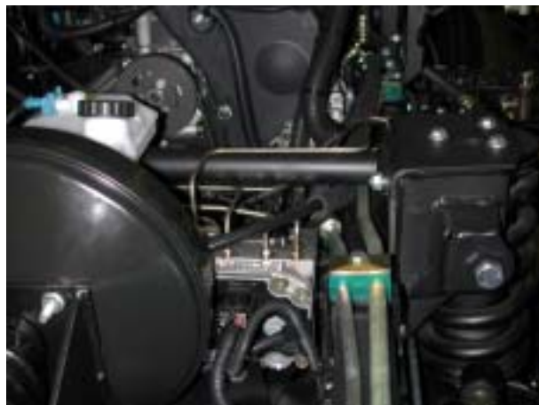
Figs. 17 and 18 Modulator installed in the vehicle's engine compartment
