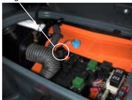
Fig. 22 Multicar switch cabinet
