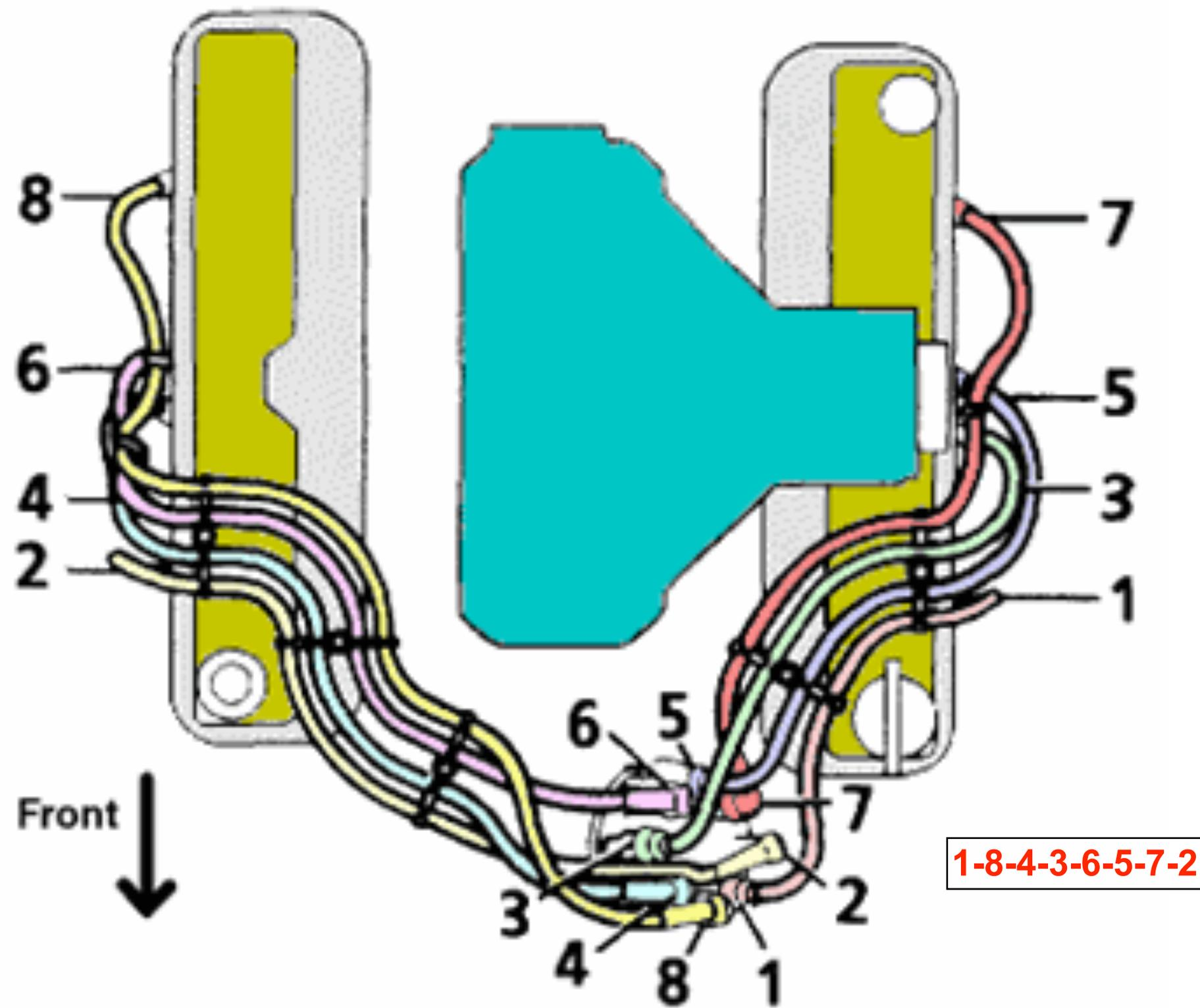
Leads 1, 3, 5, 7 are straight fittings whilst the others are 90 degree. The distributor to coil is straight with a 90 degree fitting at the coil end.
