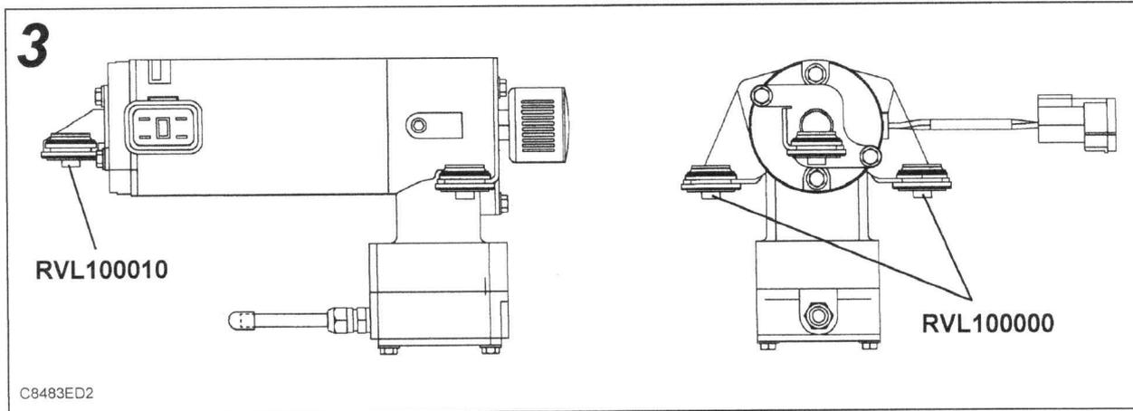
6. Refit the compressor as described in the Workshop Manual, repair number 60.50.10, ensuring that the compressor mounts are located centrally on the studs. Referring to illustration 4, refit the original dished washers 'A' and nuts 'B' to each mount, ensuring orientation is as shown. Tighten fixing nuts to 2 Nm maximum. **IMPORTANT** - do not over-tighten fixings since this will damage the new mounts.
