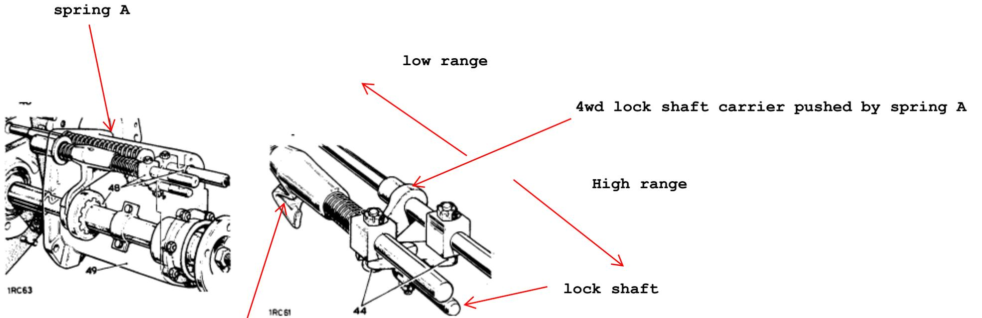
4wd selector fork/shaft forward to be engaged
