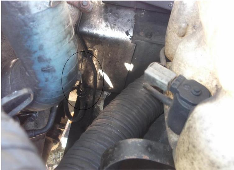
For the steering shaft, I loosened and removed the pinch bolts on the upper and lower u/j's. The shaft can then be pushed further up into the top u/j until the bottom one clears the steering box shaft and can then be removed. My lower u/j is shagged so this adds to the shopping list.
