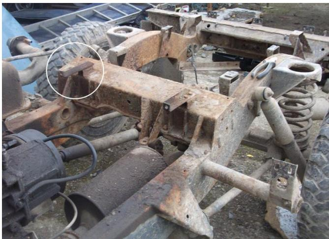
Next up, remove two bolts on each of the rear out riggers. No bother with these.
