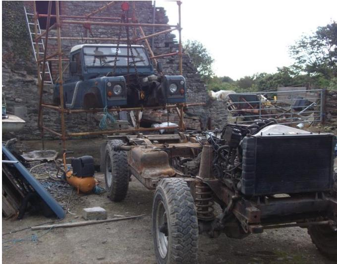
For safety I then rested the body front and rear with on scaffolding poles.
