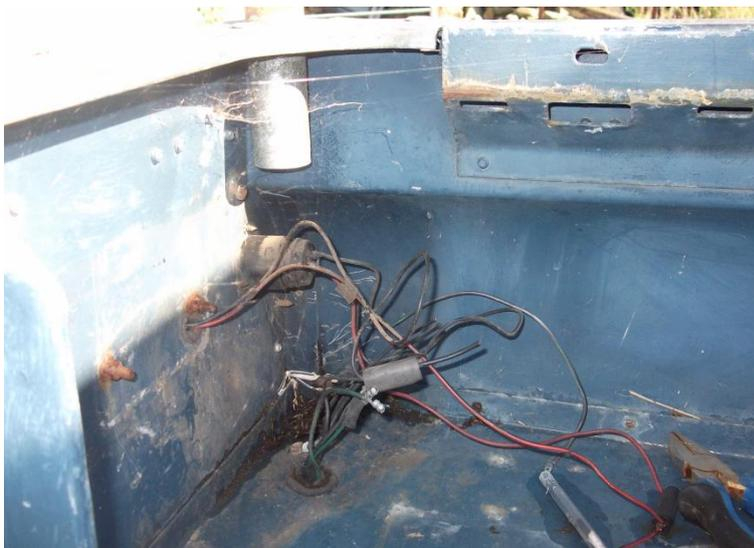
If I was doing this again I would cut the loom under the tub after it comes out of the chassis and fit a decent connection box , something like a “Rubberite” one. This would also provide a good interface for the tow bar socket.
