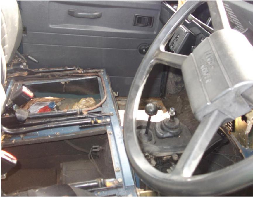
There are two bolts from the floor pan to the chassis, one each side of the gearbox, just in front of the seat box.
