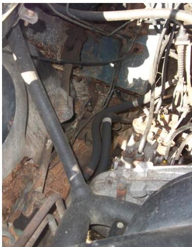
Removed the fuel filler neck from the body, this required more air chiselling as the nuts were unmoveable and inaccessible.
