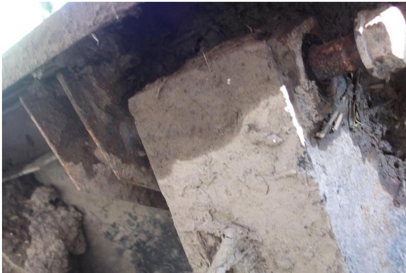
Remove the two bolts that go through the chassis legs, from the bulkhead brackets, just forward of the front outriggers.
