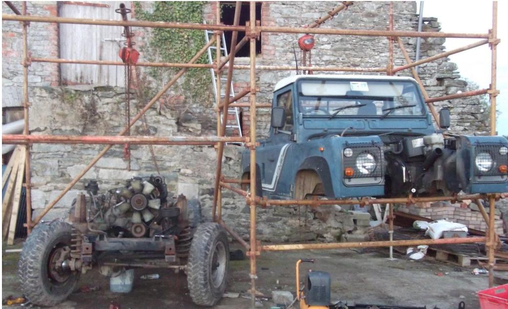
Drained the engine, gearbox and transfer box of oil ,drained and removed the radiator, connected a chain to the engine lifting lugs on the engine, and took the strain on the hoist.
