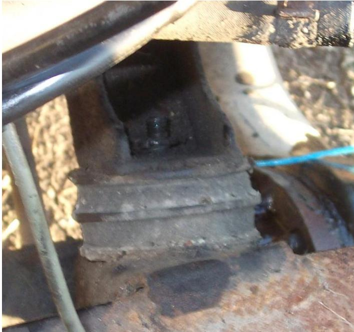
I decided to use the second hoist to support the gearbox/transfer box prior to engine lift, in case it tilted too much on its mountings during engine separation. I used a hammer and large screwdriver to carefully start the split of the engine from the gearbox.
