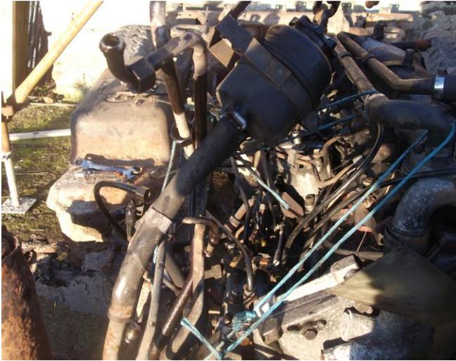
Fuel line disconnected from lift pump
