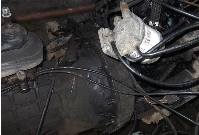
Starter and clutch slave cylinder removed.
