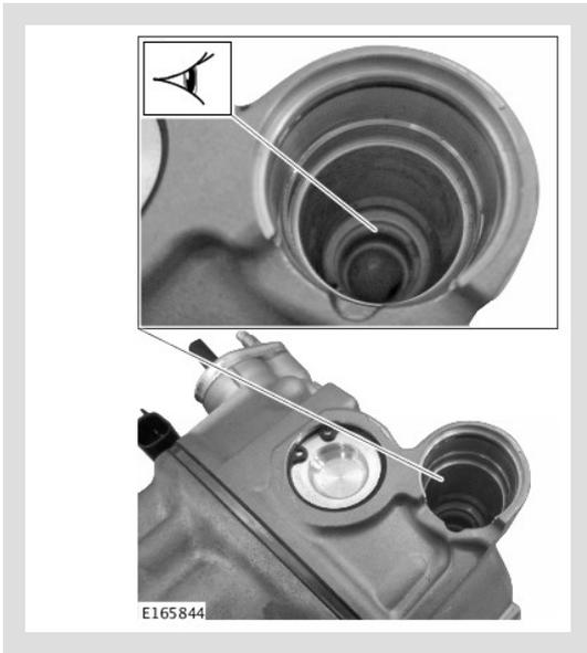
6. Apply compressor oil (Polyalkylene Glycol (PAG SPA2 Oil) to the O-rings of the new DPS valve
