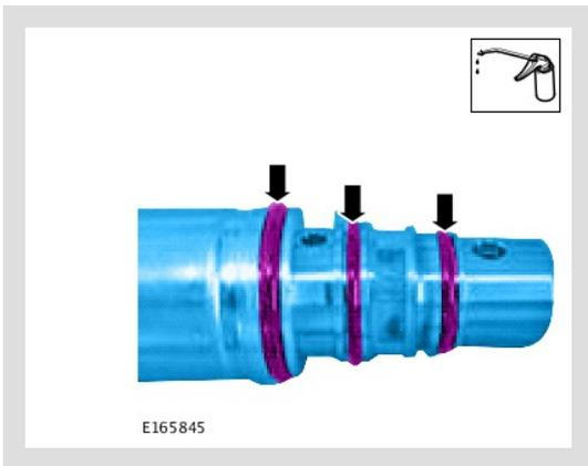
7. Install the DPS valve, apply a downward pressure by hand. Using a suitable tool if required, press fully into position to allow installation of the new circlip
