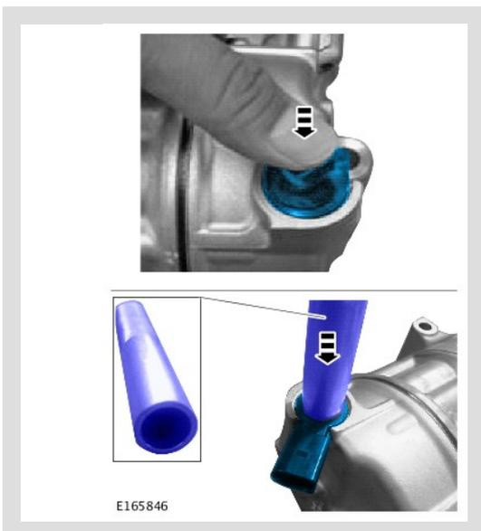
8. Using a suitable tool, install the new circlip supplied in the kit
