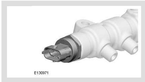
The fuel rail pressure sensor is located in the forward end of the common fuel rail for the LH cylinder bank. The sensor is screwed into a threaded port in the end of the fuel rail.
