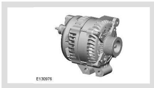
The generator has a multifunction voltage regulator for use in a 14V charging system with 6-12 zener diode bridge rectifiers.
