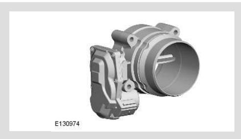
The electric throttle body is located in the intake tract to the air intake manifold. The electric throttle controls the volume of air allowed into the inlet manifold by means of a direct current (DC) motor which controls a butterfly valve in the body of the throttle. The motor is controlled by the ECM which operates the motor in response to driver inputs from the APP sensor and other engine related sensors to provide the correct air flow to the intake manifolds.
