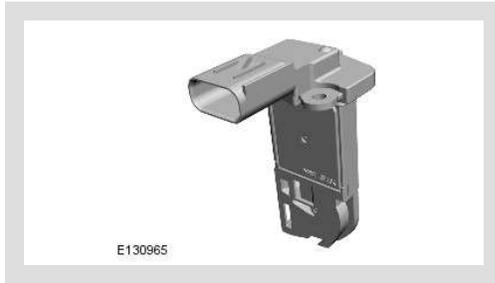
Two MAFT sensors are located on the top cover of the air filter box. The sensors are downstream of the air filters and measure the air entering the clean air ducts to the turbocharger compressors.
