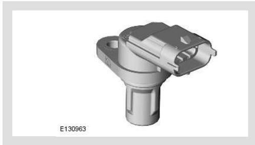
The CMP sensor is located on the rear face of the LH cylinder head. The sensor tip protrudes through the face to pick up on the reluctor behind the camshaft pulley. The CMP sensor is a Hall effect type sensor.
