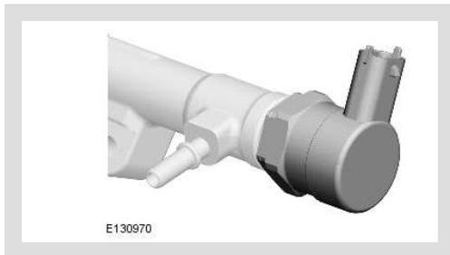
The fuel pressure control valve is incorporated into the forward end of the common fuel rail for the right-hand (RH) cylinder bank. The control valve regulates the fuel pressure within the fuel rails and is controlled by the ECM. The control valve is a PWM controlled solenoid valve.
