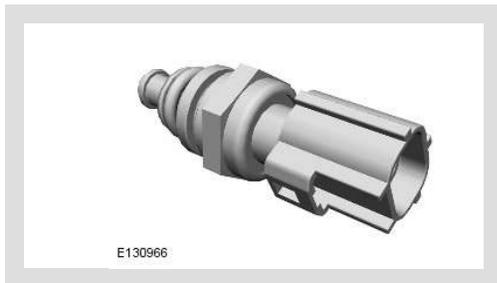
The engine coolant temperature (ECT) is located in the thermostat housing. The ECT sensor provides the ECM and the instrument cluster with engine coolant temperature status.
