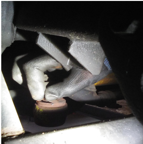
Fig 4 - Supporting Image Check gear box fluid level manual / automatic differential (If applicable)
