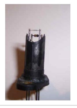
To test the air flow sensors output, connect the meter between the the ground (red black wire )and air flow sensor output (blue green wire). By removing the air filter and looking into the mouth of the air flow meter, a small hole will be seen in a cutout that runs around the edge of the air intake. By blowing gently into this hole the voltage should rise sharply on the airflow output. Not a scientific calibration, but a basic confidence check.
