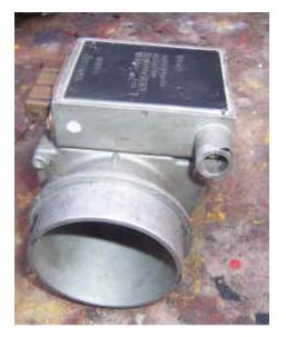
Applicable to NON catalyst cars only. Using a voltmeter between red and black wire and blue and red wire check the voltage with the ignition on, but the engine not running. Recessed Hex head screw allows you to set the carbon monoxide base line with these voltages. NOTE these are base settings ONLY. Turn the adjustment screw clockwise to richen the mixture, and anticlockwise to lean the mixture. The screw has multiple turns, that will go from 0 volts to over 3.5 volts.
