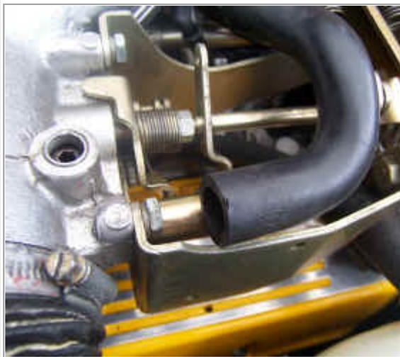
Remove this pipe from the plenum chamber, and insert the sealing plug to make an air tight seal. Refit the pipe to prevent air reaching the air control valve.
