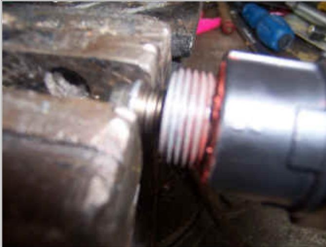
Clamp the cone securely, then rock the motor side to side and pull.
