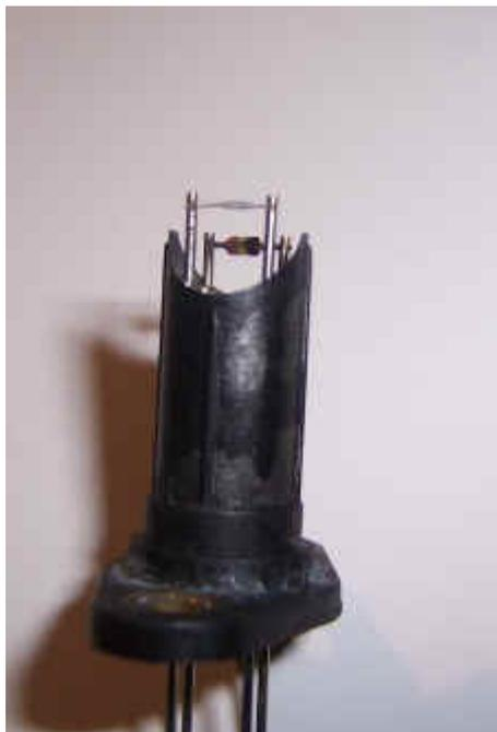
This is the hot wire sensor (enlarged). The grey sensor in the foreground is the actual hot wire sensor, with a temperature sensing thermistor behind it. The hot wire can get coated in road dirt, that changes its cooling characteristics and causes the output from the AFM to be incorrect. It is difficult to clean without removal, although a blast of "easy start" or the like might be enough. Removal requires a complete strip down of the AFM
