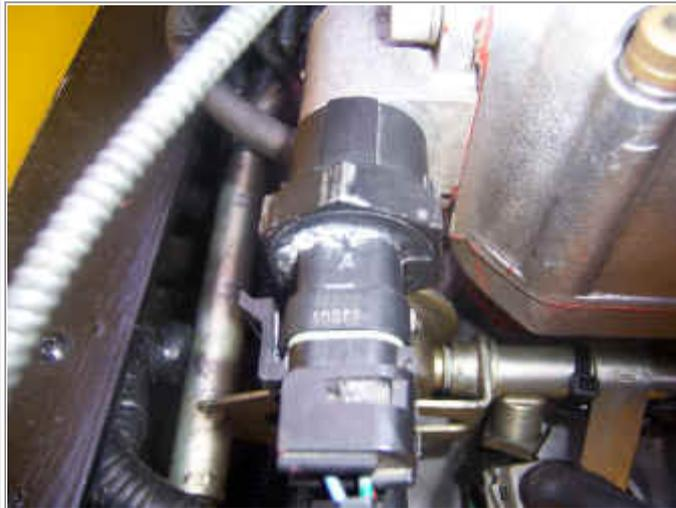
Air control valve. This comprises of a stepper motor, with a worm drive that moves a conical valve to control the amount of air by passing the throttle butterfly, and hence the tick over. Very prone to sticking, leading to erratic tick over.
