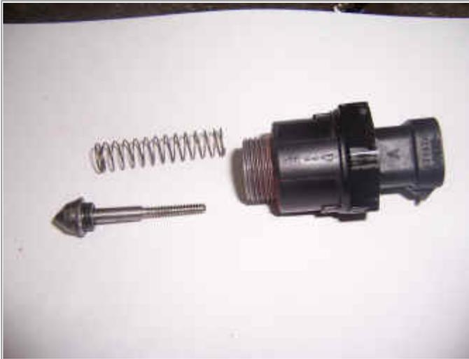
The component parts. Clean the cone, shaft and keyway.
