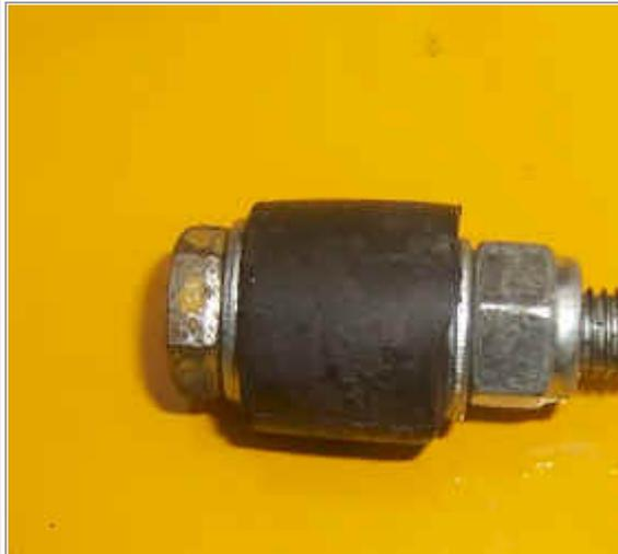
Make up a sealing plug with a M6 bolt and a bit of fuel hose. Tightening the bolt will expand the hose to provide a good seal (see below).
