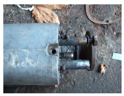
Video of selector shafts movements not mine https://www.youtube.com/watch?v=Jz9uvVRFywk Transfer box selector shaft measurements in various positions as below.
