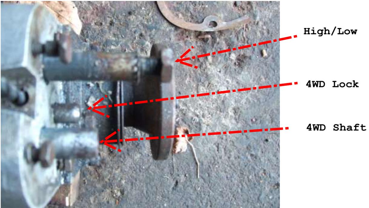
High 4wd      high/low 68mm      4wd lock 27mm      4wd shaft 51mm
