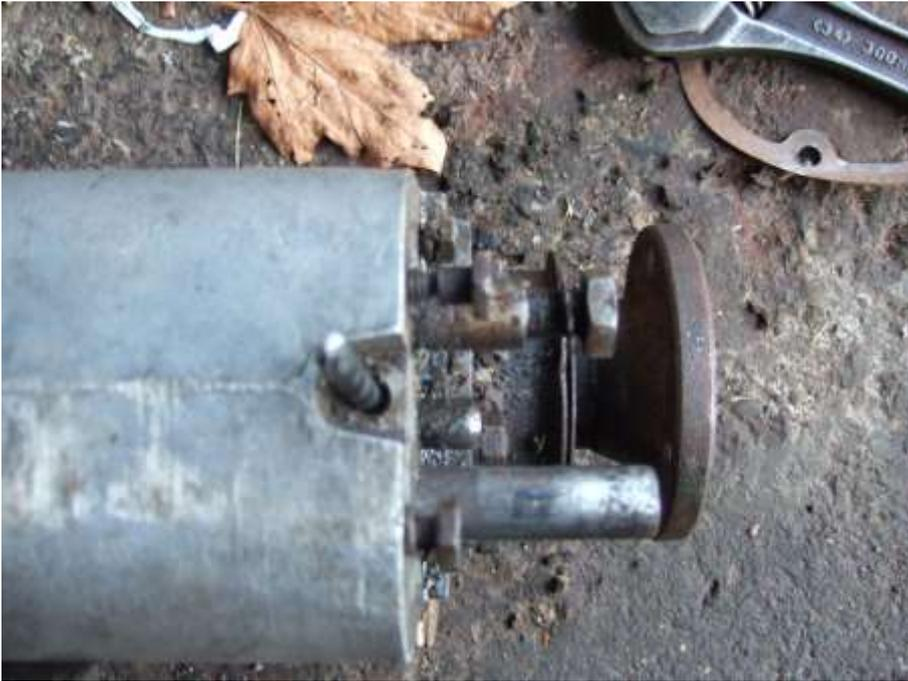
Neutral high/low lever 56mm      4wd lock 15mm      4wd shaft 44mm
