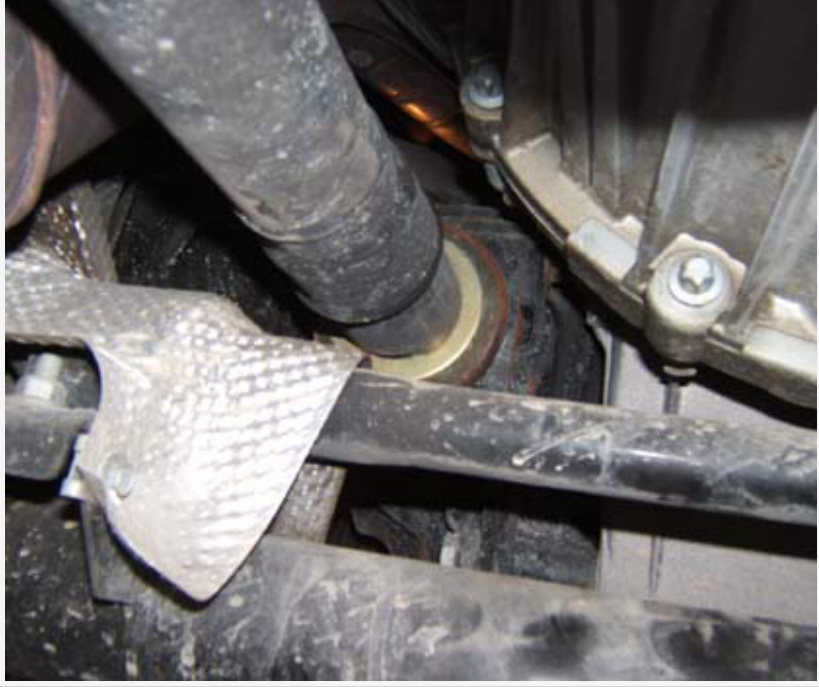
Front end of original driveshaft, where it enters the front diff, without flex coupling of any kind.
