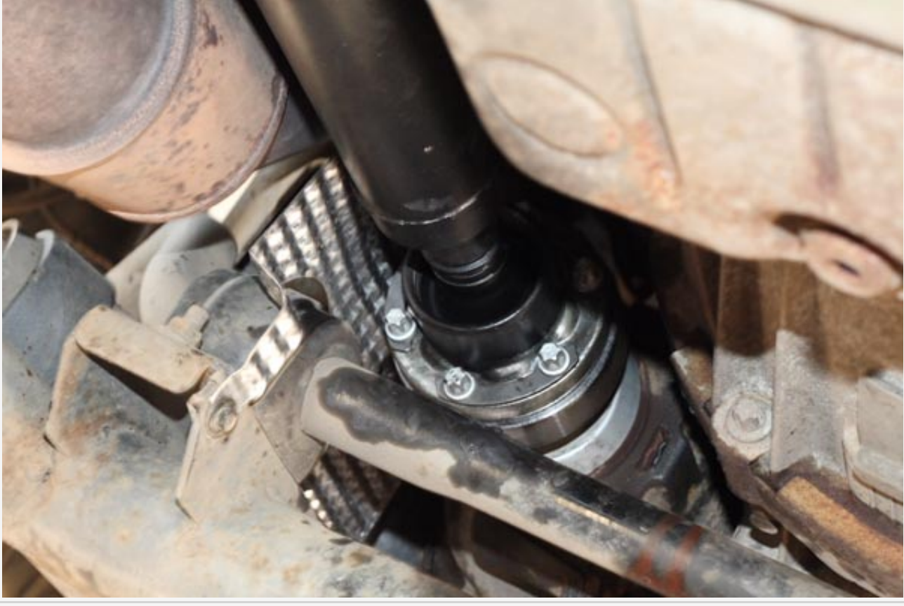
Flexible coupling at front end of new driveshaft for 2003-2005 models. Note resemblance to 2006 design. Note new heat shield, also installed as part of the service action, to the left of the drive shaft to shield it from the catalytic converter.
