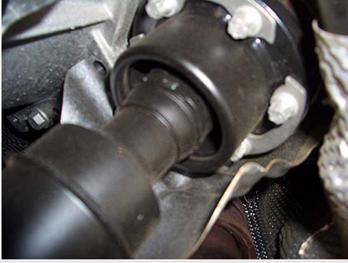
Flexible coupling used on front end of redesigned drive shaft for 2006 and up models with Jaguar-derived engine.
