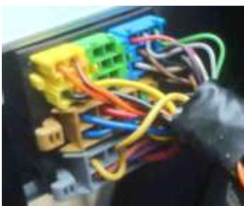
(Sorry, no pic of the red mini-ISO housing that that connector plugs into!) The pins should 'click' home when the locking tabs engage.
