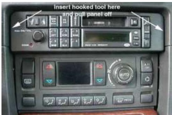
MY '99 onwards – A few changes were introduced. Firstly, the HUs and CD changers were now manufactured by Alpine, and some changes were made to the wiring harnesses. In addition, the system may have a single 'DSP' amp that lives behind the soundproofing behind the subwoofer unit in the boot – OR it may still have the door amps setup. Alpine HUs on the Harman / Kardon systems mostly look like the following picture (although there are some variations about):
