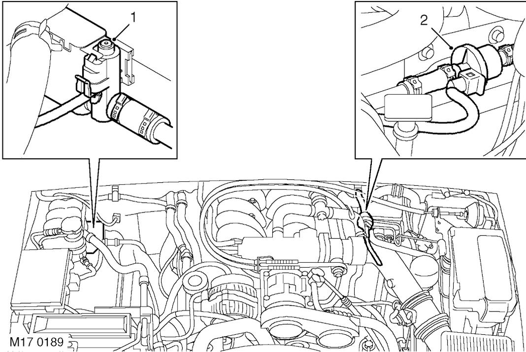
1. Canister Vent Solenoid (CVS) unit - (NAS only)
