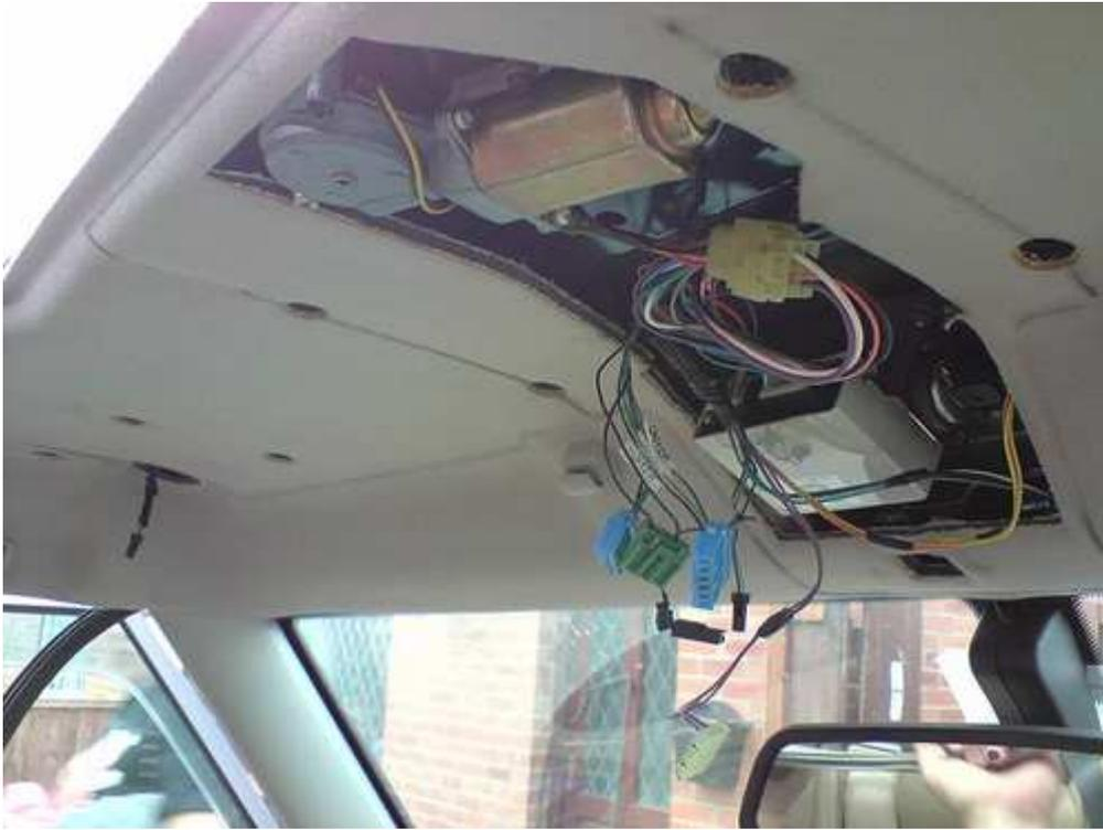
Now, pull the rear of the headlining down and put the dickie seat headrest back up and you can then withdraw the headlining out the back door.
