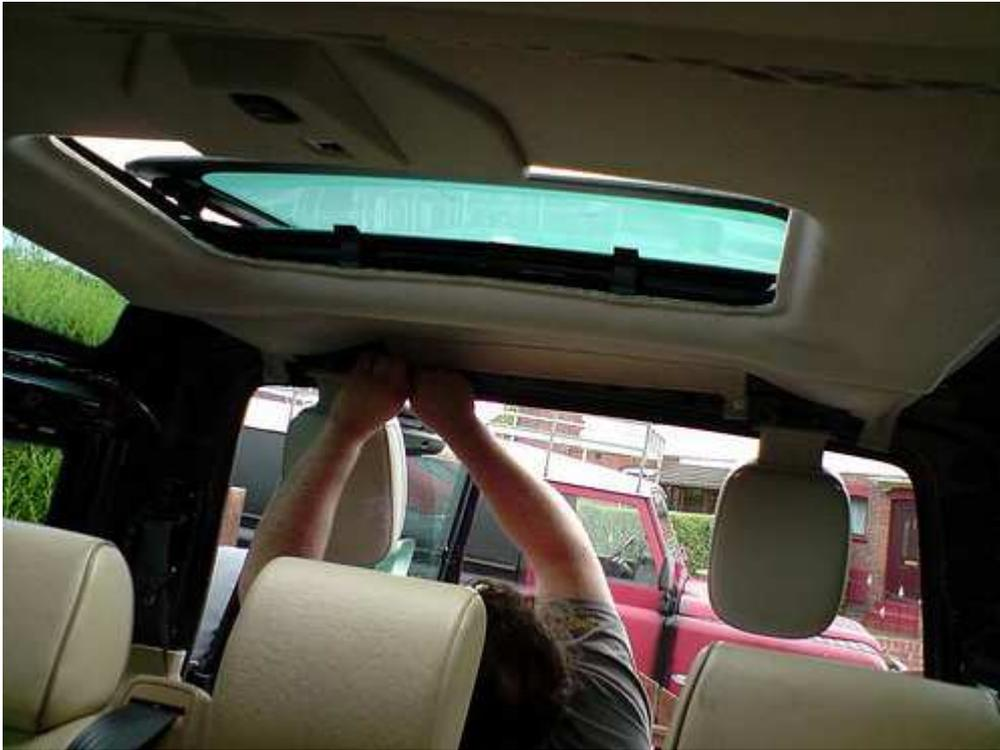
Once thats off, move on to the main side rear panels. These are held on by a combination of 5 long plastic pushclips and 2 little screws under plastic covers. The covers snap off really easily so be careful. then just pull off the alarm motion sensor, its held on by 2 metal friction clips and comes off easy enough.
