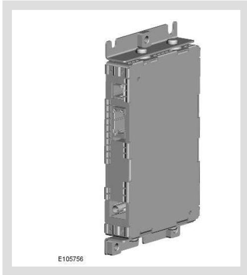
The SDARS receiver is a dedicated SDARS head unit and tuner which is controlled by the IHU on the MOST ring. The receiver is located in the LH rear of the luggage compartment.
