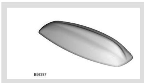
The SDARS antenna is located in the roof pod and is shared with the telephone system and the navigation system where fitted. The roof pod is located externally in a central position towards the rear of the roof.
