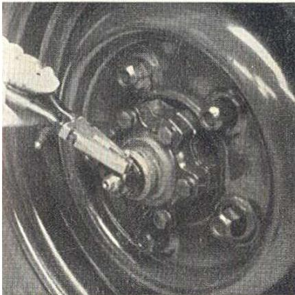
2. Remove the cotter pin securing the castellated nut on the extension of the stub axle.
