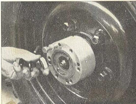
7. Fit the new rubber and felt oil seal with washer on the splined stub axle and screw on the original castellated nut. **DO NOT OVERTIGHTEN**, i.e., first tighten the nut and turn back to the nearest position for the cotter pin to be inserted and spread.
