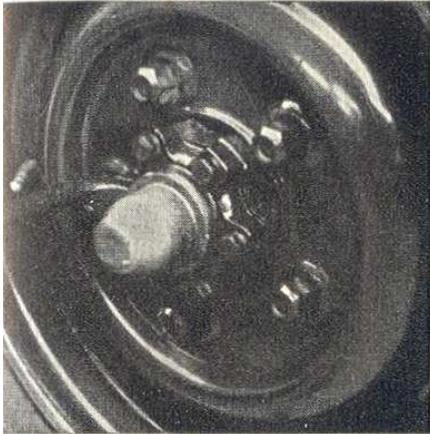
1. Remove the oil cap covering the extension of the front stub axle.
