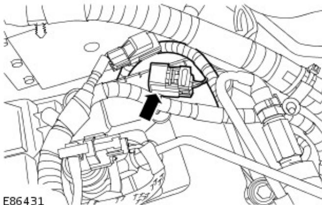
4. Using the special tool, remove the CHT sensor.
