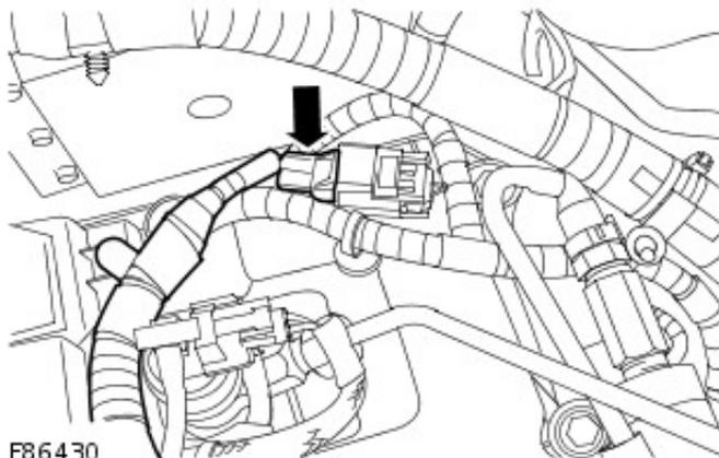
3. Release the CHT sensor wiring harness.
