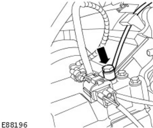
**14.** Disconnect the transmission range selector warning lamp electrical connector.
