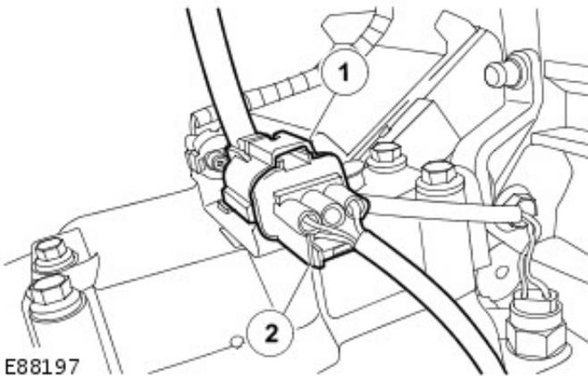
**15.** Disconnect the differential lock detection switch electrical connector.
