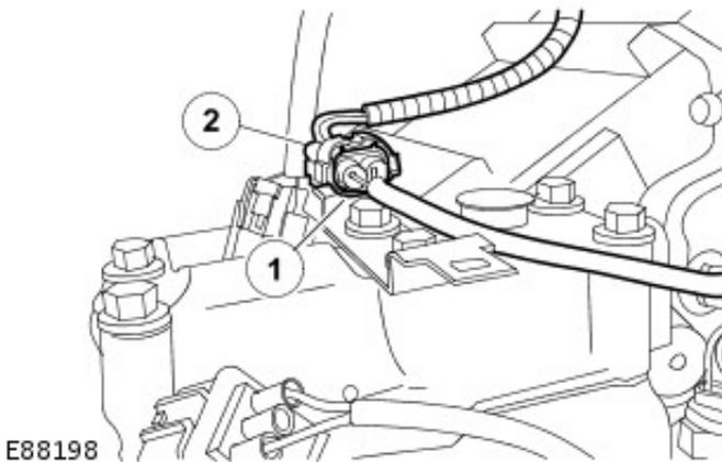
**16.** Disconnect the transmission range selector rod.
