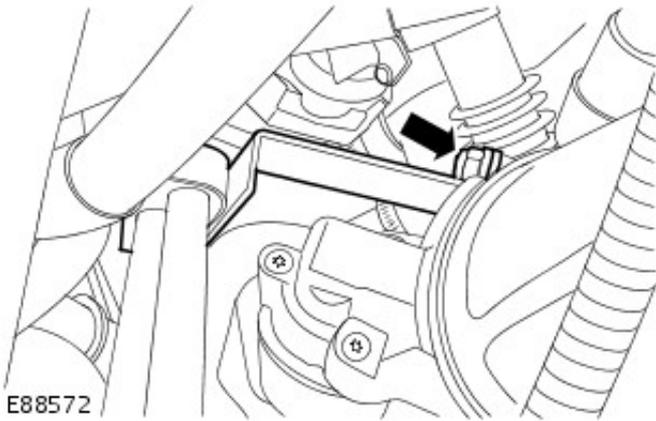
6. Connect the battery ground cable.
