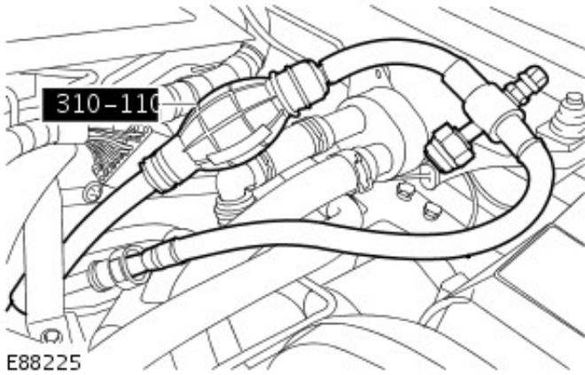
4. Connect the fuel injection pump supply line.
