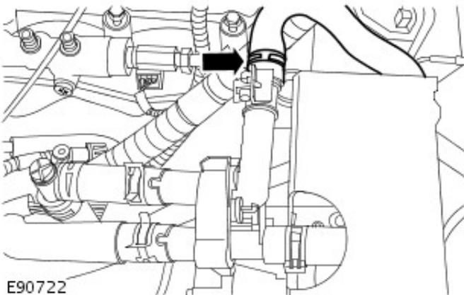
4. Disconnect the heater control valve feed and return hoses.
