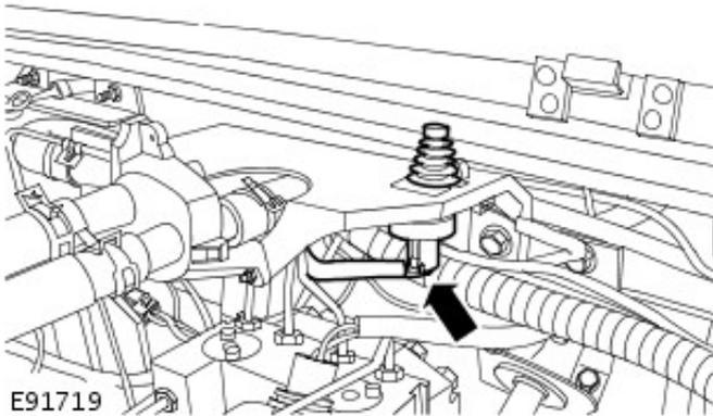
2. **NOTE:** Note the fitted position of the cable prior to removal.
