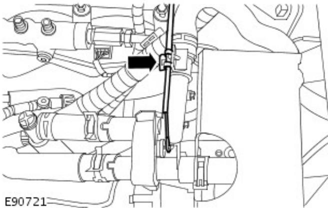
3. Disconnect the heater core feed hose.
