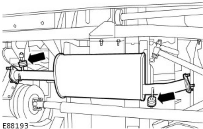
6. Remove the intermediate pipe and muffler.
