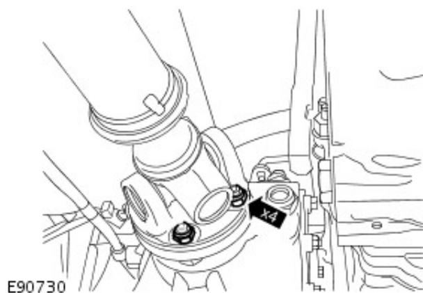
7. **NOTE:** Mark the front driveshaft to transfer case drive flange.
