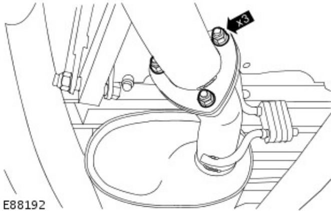
5. Release the tail pipe from the intermediate pipe.
