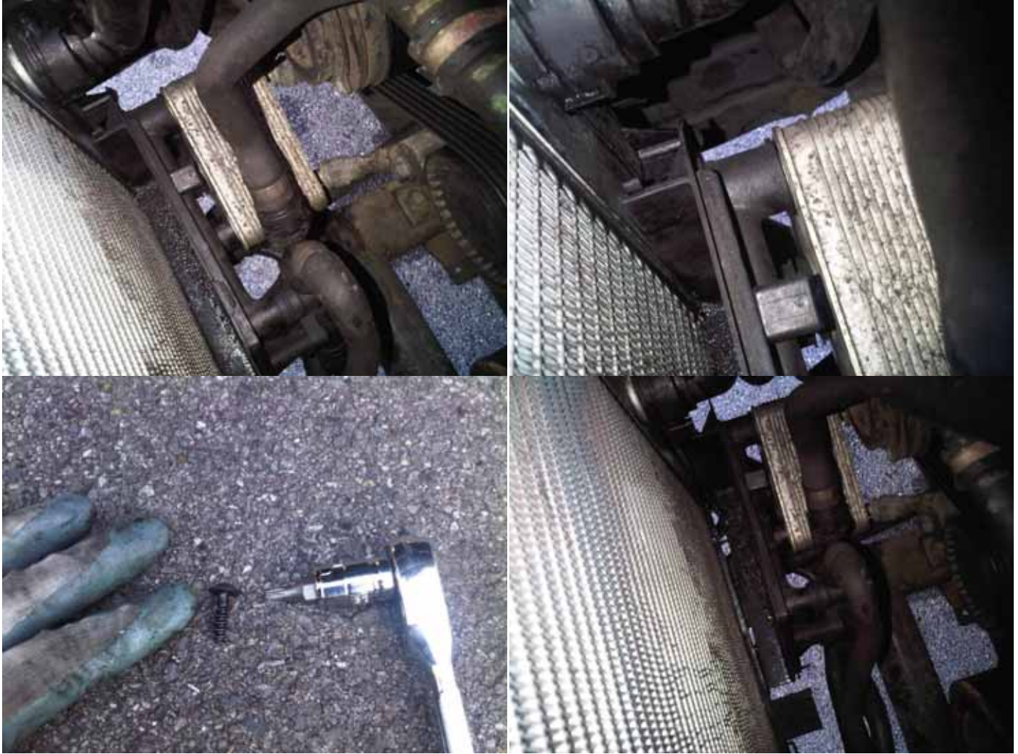
The 4 Pipes attached to the Rad – Bottom Hose, Bypass Hose(?), Top Hose and Expansion/Bleed Hose.
