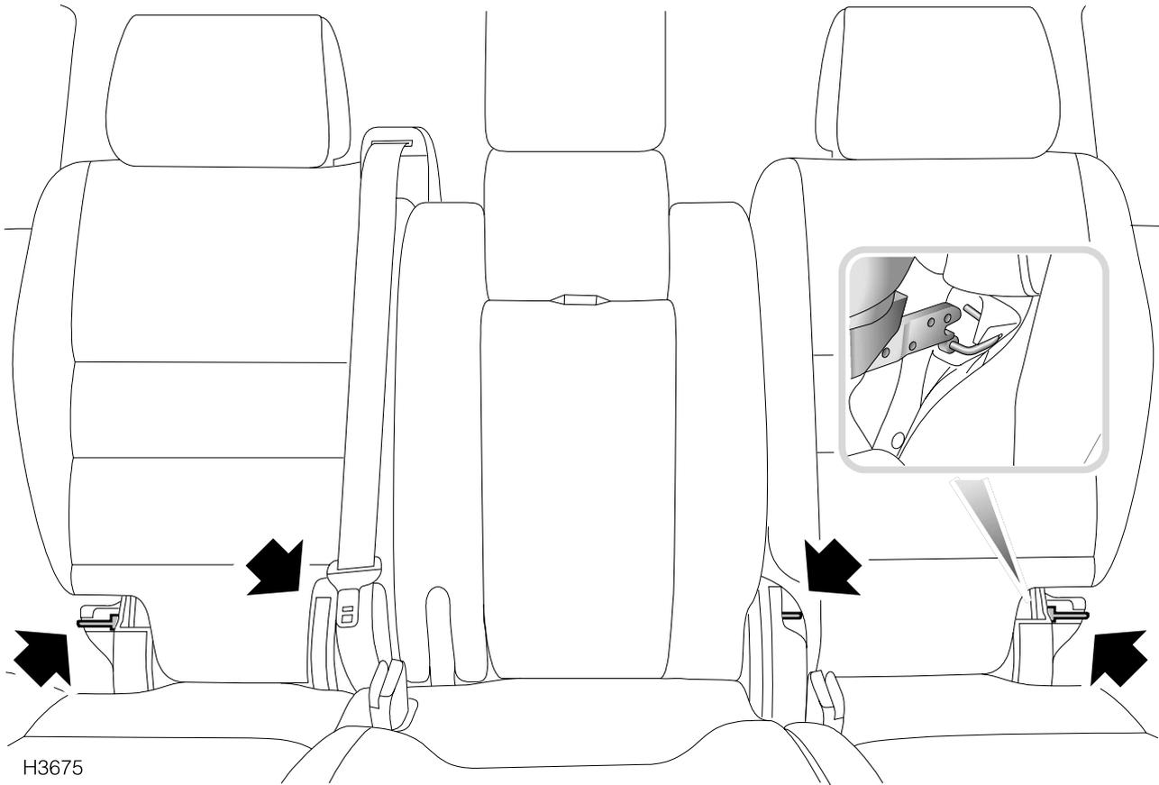
In some markets, child restraint systems complying with International Standard Organisation (ISO) regulations and approved for fitting in your vehicle may be available. These restraints are different to conventional child seats, requiring anchor bars built into the vehicle seat in order to accept the ISOFIX locking mechanism.
