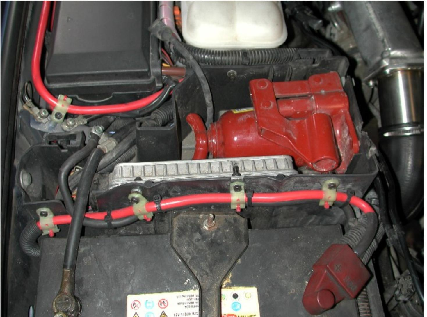
*Here because of my winch install, I had to remove the "p" clips holding the power cables going to the winch as they also hold the ECU. Your ECU "should" be held by just 1 self tapping screw, which you can remove, also lift out the bottle jack and put aside to give you more room as well.*
