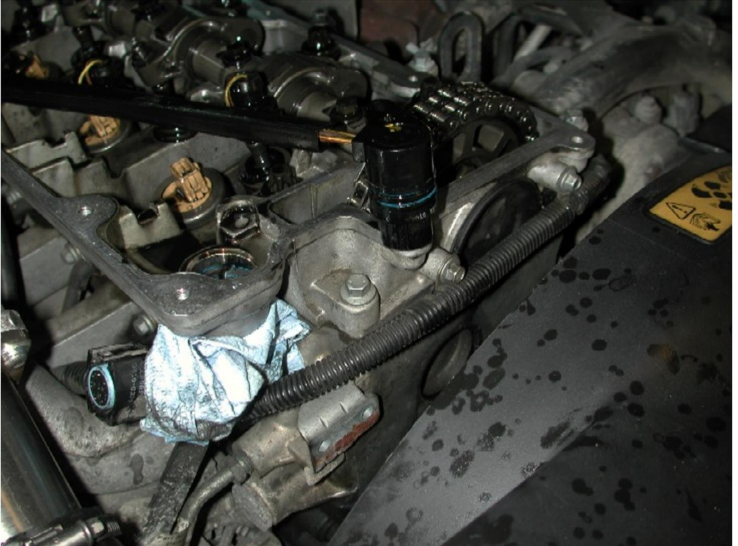
*And the plug that is underneath where the main loom joins the injector harness. Once they are all disconnected, the harness simply lifts out. Below you can see the 2 guilty "o" rings that fail and allow the oil to pass into the loom.*
