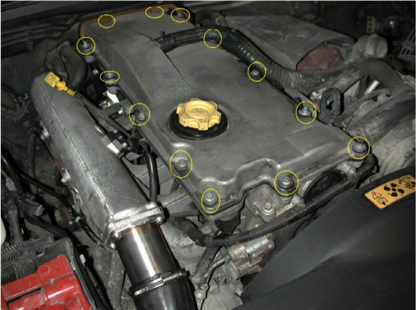
*The bolts have bushes and rubber washers on each one, so make sure you collect all of them before lifting the cover off.*
