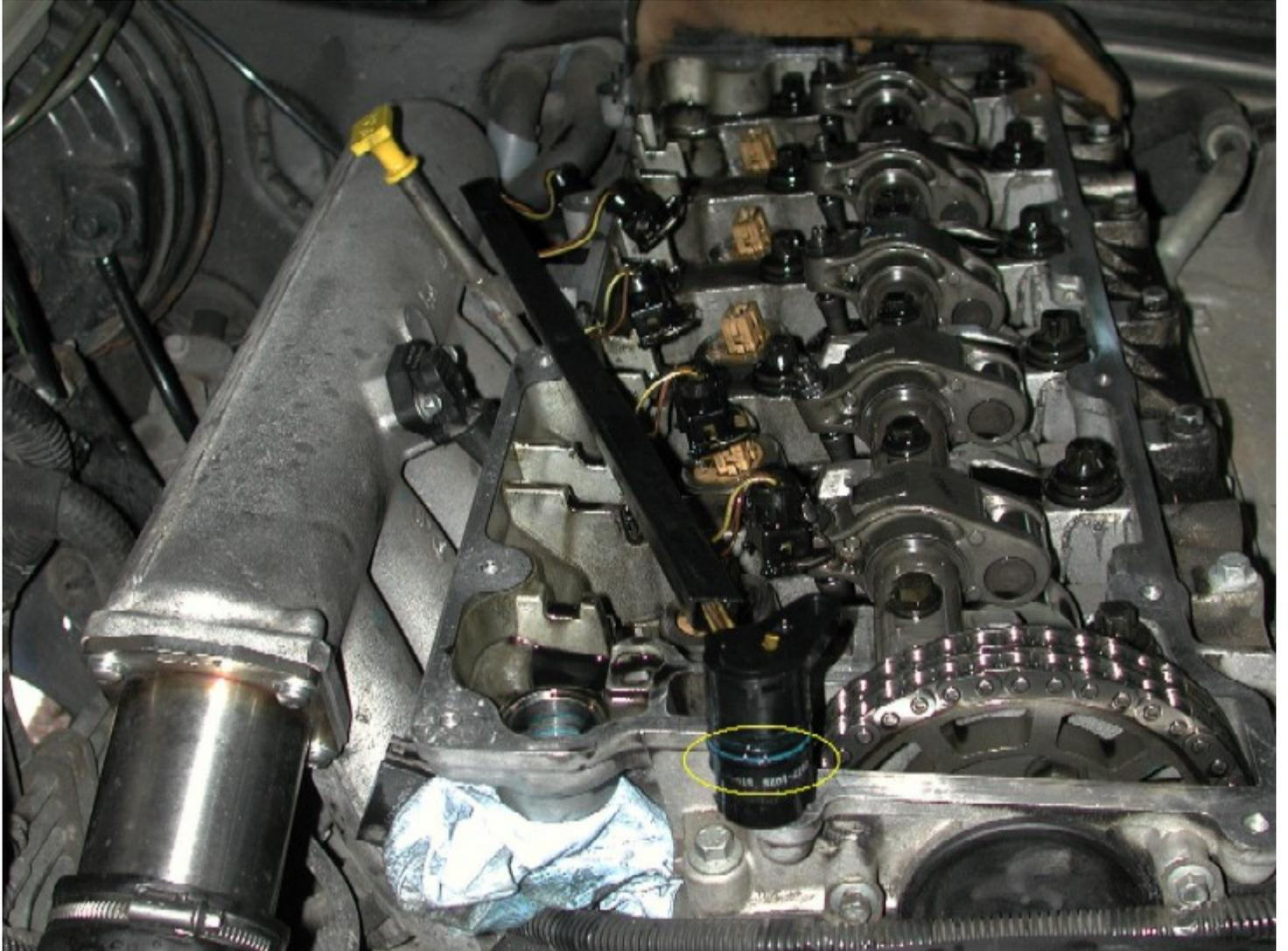
*You can also see above where the "o" rings have stuck themselves in the hole to the head, this ideally needs to be cleaned up before fitting the new one, use some scotch bright pads or "very" fine emery paper to carefully clean up the hole where the plug sits.*
