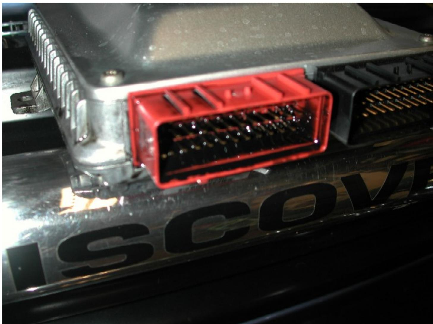
*As you can see, the RED plug socket is full of oil, It was probably only a matter of time before it may have began to give me rough running issues. Below you can clearly see the oil has got to all parts of the plug as well....*
