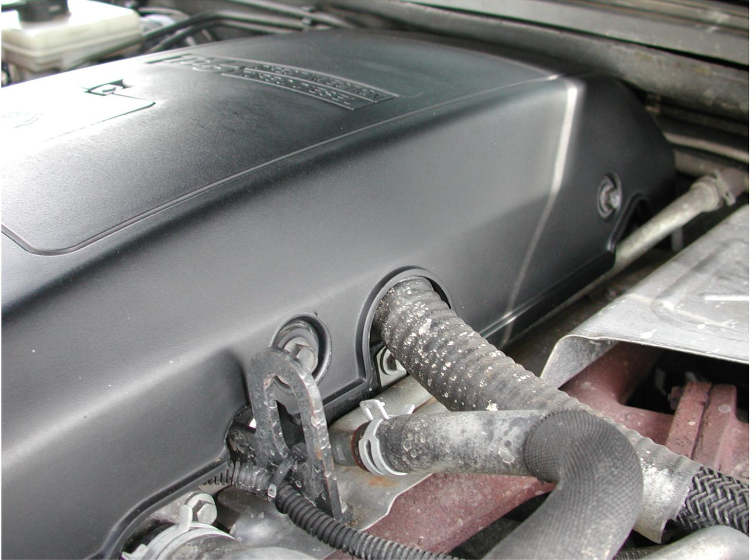
*Next remove the battery cover, and disconnect the battery earth lead as this will be needed to be moved out the way to allow you to remove the ECU.*
