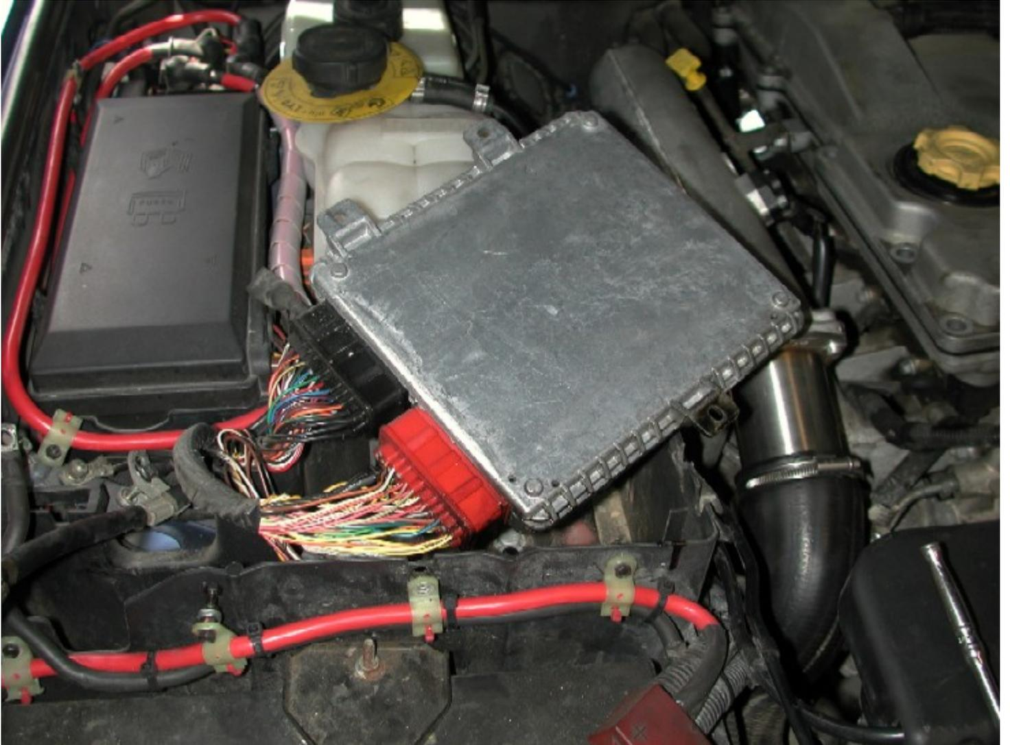
*Now you can lift out the ECU, Here in the pictures you can see the "small" amount of oil I had noticed on the bottom of the RED plug, from looking at it when the ECU is installed.*
