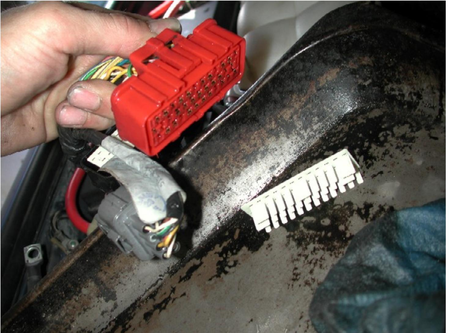
*I used a fast drying solvent spray to clean all the oil out of the plug, and left it to dry / drain whilst I went onto the next bit. You will also see an orange rubber seal inside the plug, you can carefully "hook" that out to clean that as well. With the amount of oil that was actually in the plug, I was unsure whether or not it had actually made its way into the ECU itself.*
