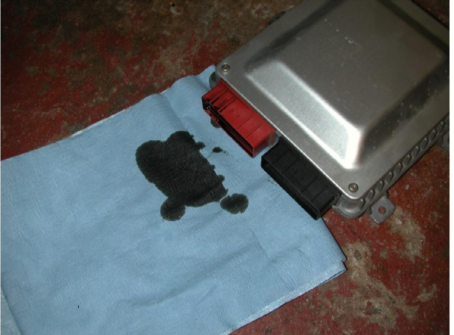
*With this in mind, I decided to remove the top cover of the ECU to have a look inside to see if that was ok, The cover is held on with 4 tamper proof torx bolts, the top is also sealed / stuck down and needed to be levered free VERY carefully. The top is only thin aluminum, so if you go at it to hard you WILL damage / bend it out of shape. "If" you decide to take the ECU top of, do it entirely at YOUR OWN RISK.....*
