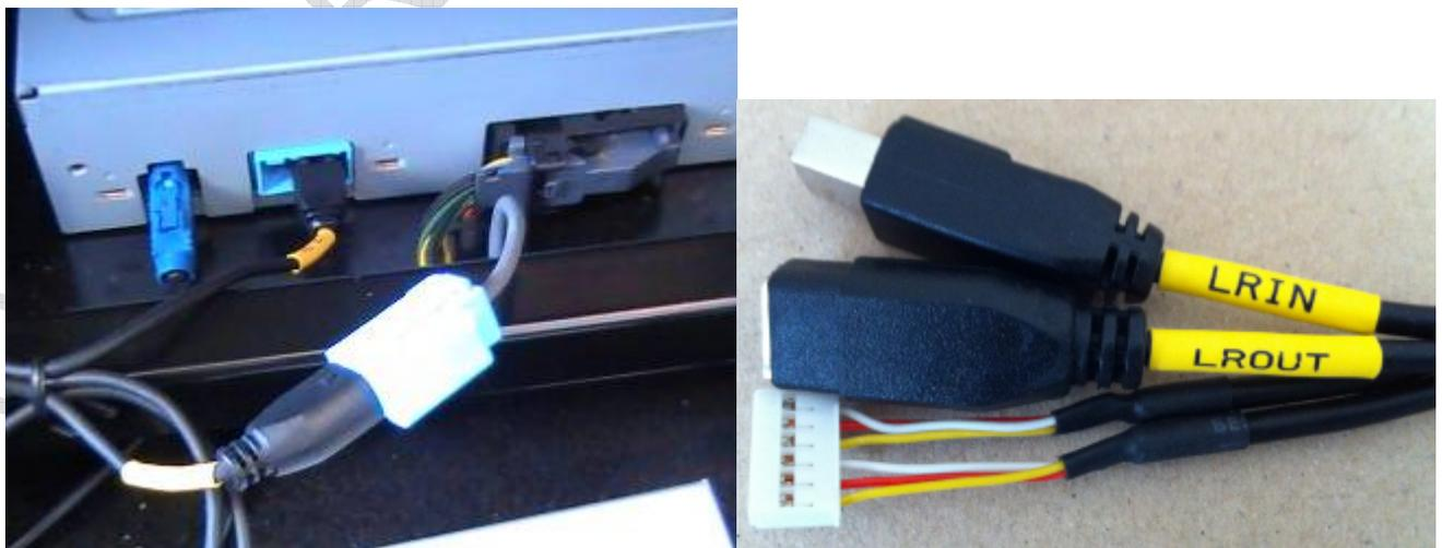
4. Connect the 12volt positive and negative supply to the main wiring harness of the GVIF unit – these are the red and black cables coming from the filter/fuse part of the harness and also the green cable to earth as shown below:
