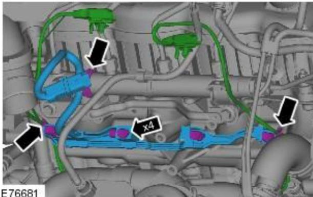
Remove the LH and RH glow plug wiring harnesses.
