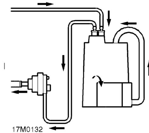
When the temperature of fuel in the tank reduces, pressure also reduces and vapour must be drawn back into the tank. Fresh air is drawn into the canister, through the open vent solenoid, to take up the displaced volume.
