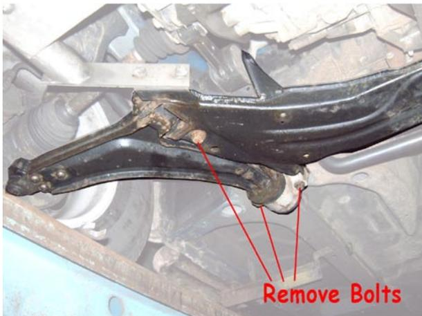
3 Slacken the bolts (on both sides of the vehicle) as shown in the picture above. The Sub frame and wishbones should now all be loose and you should be able to remove the anti roll bar. The fitting of the new anti roll bar is the reverse procedure. Ensure all nuts and bolts are tight before driving the vehicle.
