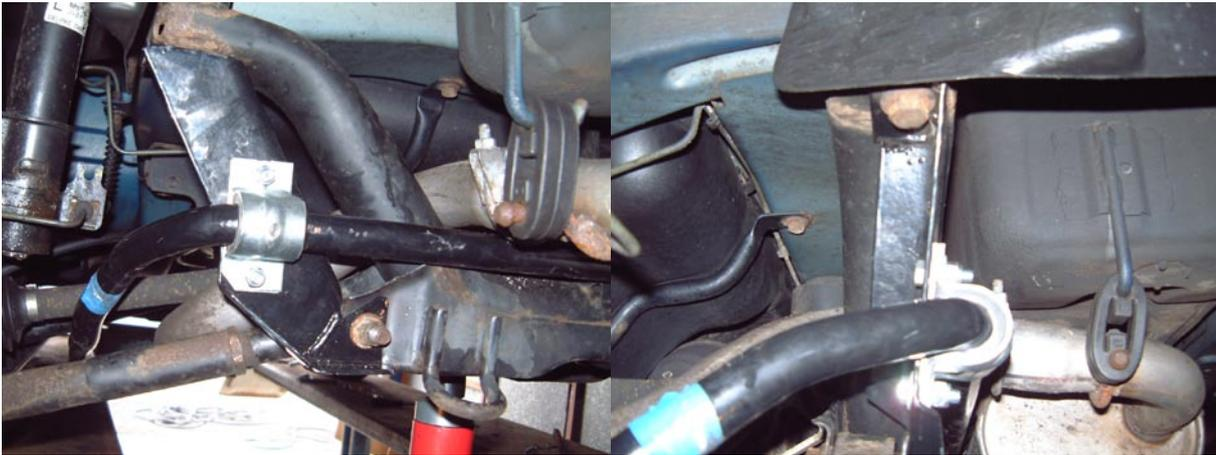
2 It should be routed under the rear drive shaft but over the rear adjustable suspension link assembly. The ARB then bolts to the front of the rear shock/strut assembly using the brackets supplied. Don't forget to re tighten all nuts and bolts which have been loosened, including the exhaust, before driving the vehicle.
