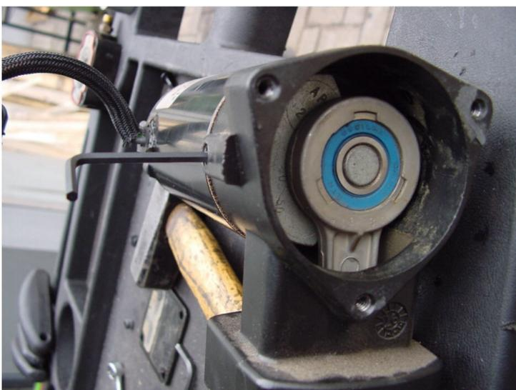
**9.** Unscrew head screw from the piston (wrench #3 or #3.5)
