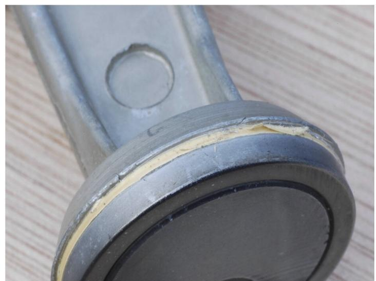
**10.** Take the piston out of the crankshaft. Use a screwdriver to loosen it, if applicable..
