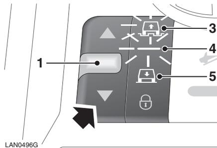
When Extended mode is activated, indicator (3) will flash if the suspension is above Off-road height. Indicators (3) and (4) will flash if the suspension is between Off-road and On-road heights. Indicators (4) and (5) will flash if the suspension is between On-road and Access heights. A message will be displayed on the message centre.
