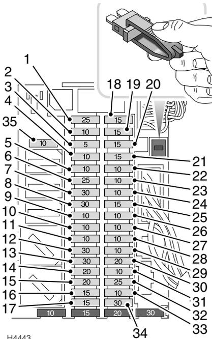
Press the fuse removal tweezers onto the head of the suspect fuse (as shown) and pull to remove. A break in the wire inside the fuse indicates that the fuse has 'blown' and must be replaced.
