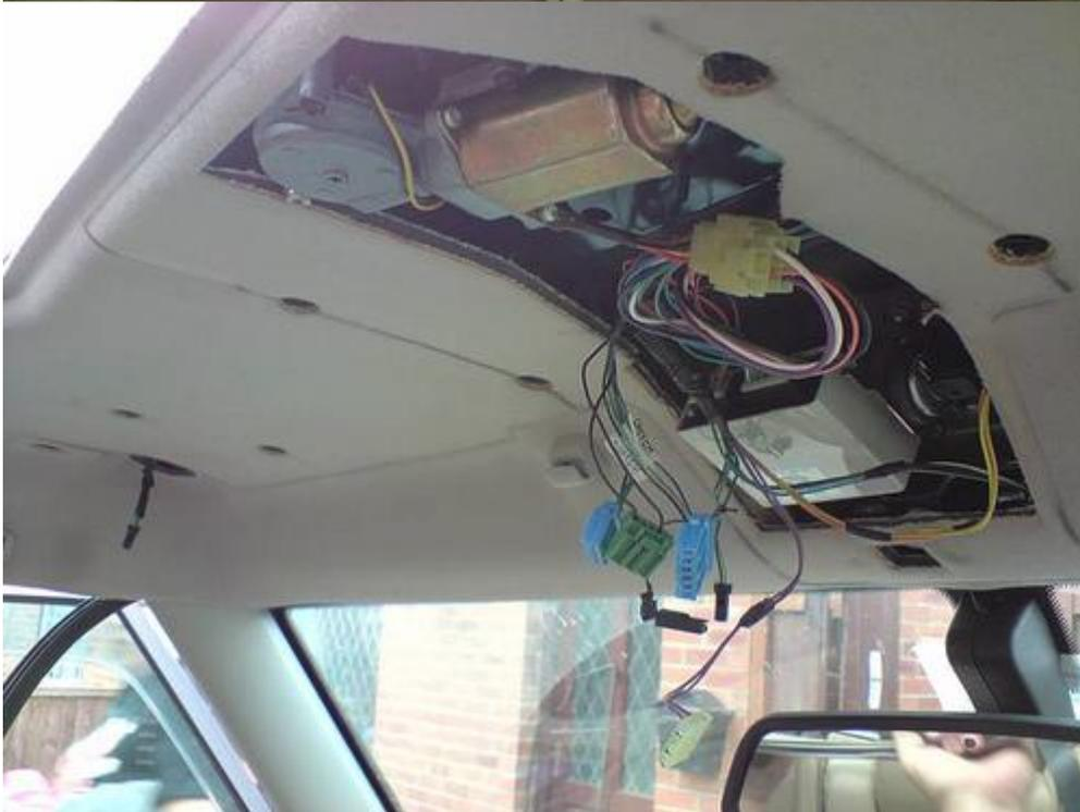
Now, pull the rear of the headlining down and put the dickie seat headrest back up and you can then withdraw the headlining out the back door. It is a tight squeeze and does involve a bit of pushing and shoving and gentle bending. Dont worry about creases, as long as you dont go overboard no permanent creases will remain in the fabric or fibreglass headlining.
