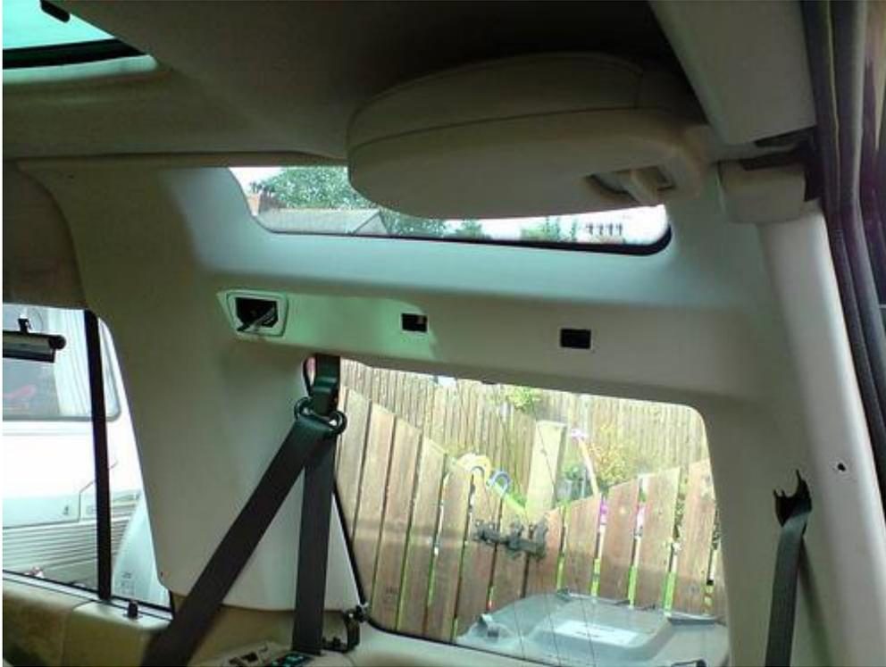
Now the only thing stopping you removing the panel is the rear dickie seat 3 point seatbelt. Remove the 17mm bottom anchor bolt and then remove the plastic trim covering the whole in the panel that the belt feeds through, there should now be enough room to feed the belt and clip through the hole and the rear panel should now be free,
