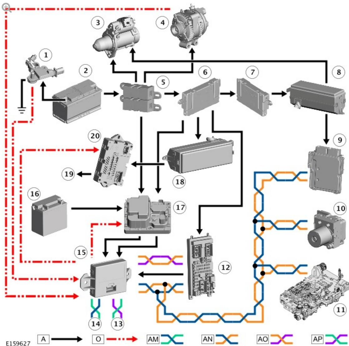
A = HARDWIRED; O = LIN BUS; AM = HS (HIGH SPEED) CAN CHASSIS BUS; HS CAN POWERTRAIN BUS; AO = MS (MEDIUM SPEED) CAN BODY BUS; AP = MS CAN COMFORT BUS.
