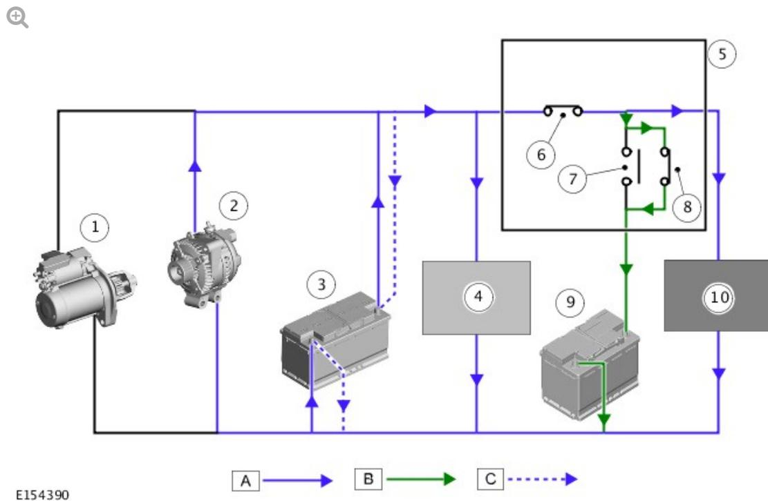
A = PRIMARY BATTERY/GENERATOR SUPPLY; B = AUXILIARY BATTERY CHARGING; C = PRIMARY BATTERY CHARGING.
