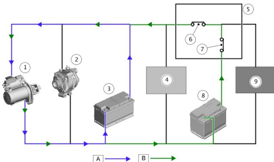
NOTE: A = PRIMARY BATTERY SUPPLY; B = AUXILIARY BATTERY SUPPLY.
