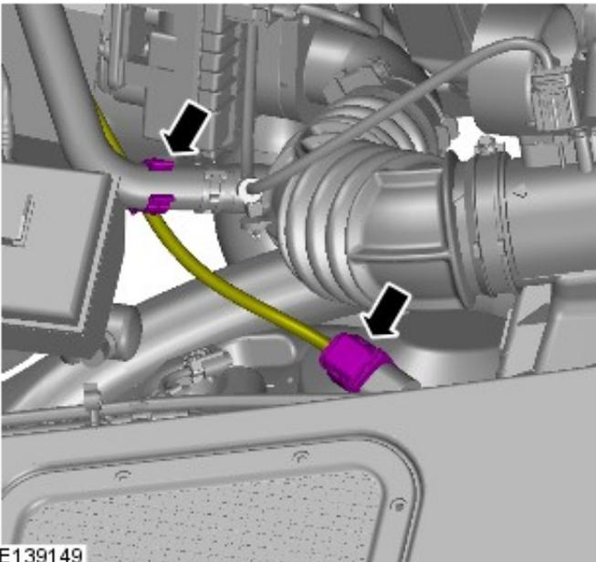
3. Torque: 48Nm Tool: 310-121 (Wrench, HO2S)
