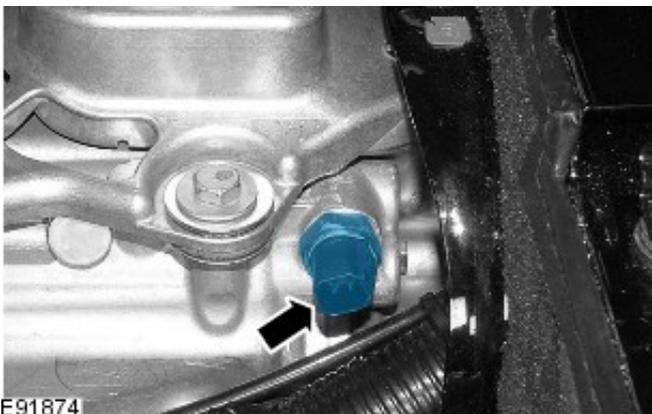
2. Connect the reversing lamp switch electrical connector.
