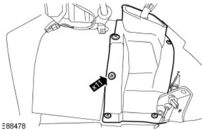
10. Disconnect reversing lamp switch connector.
