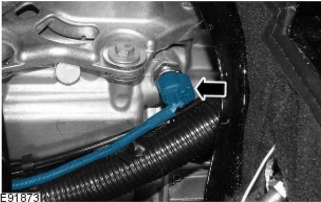
11. Remove the reversing lamp switch.
