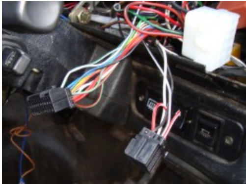
New warning panel plugs being wired in
