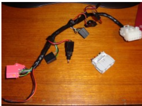
The finished loom, taped back up and ready for fitting
