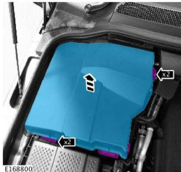
5. Remove the retaining nuts and position the electrical wiring to one side.
