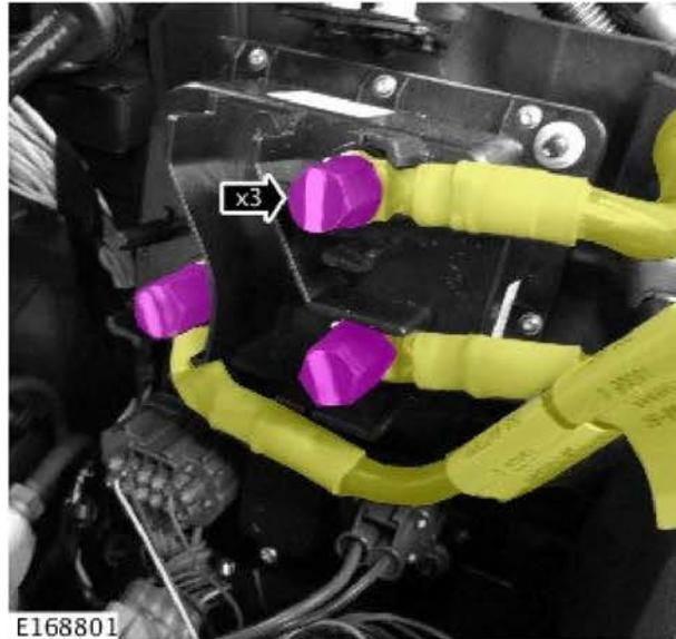
6. Disconnect the electrical connectors and position the electrical wiring harness to one side.
