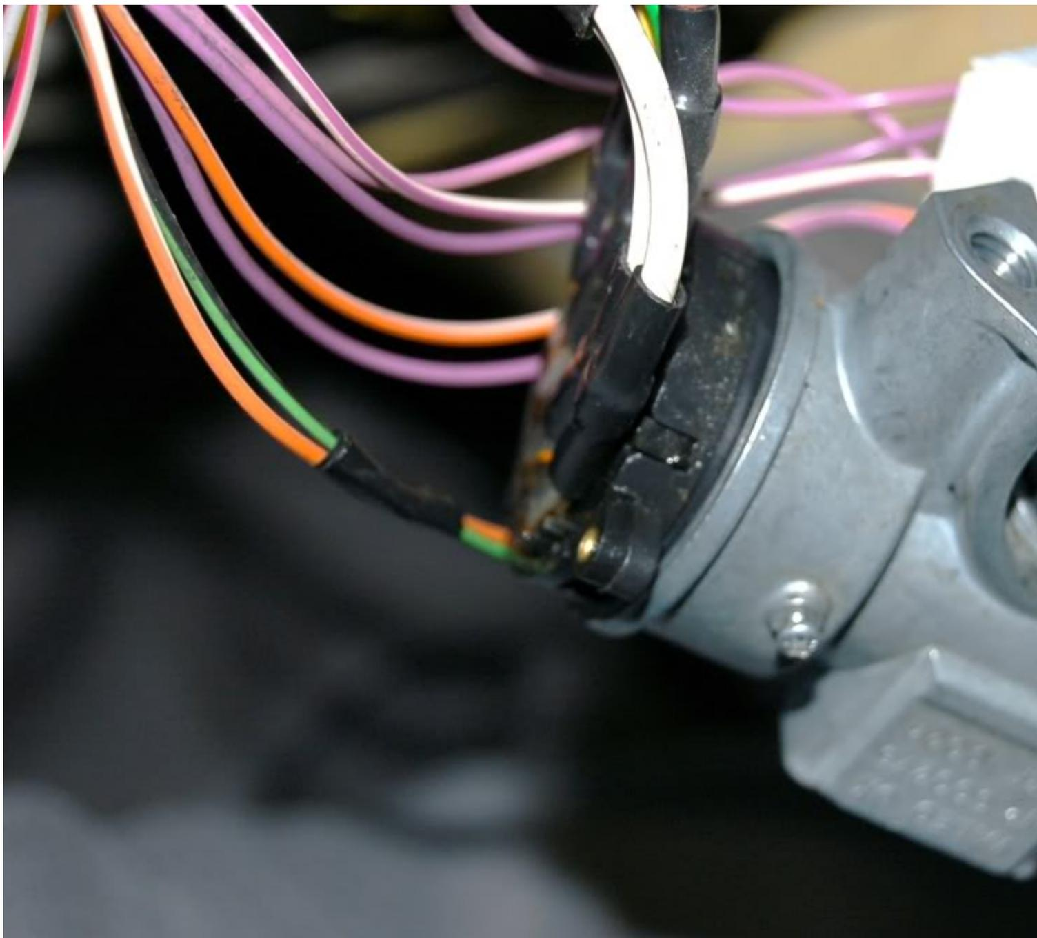
...unplug rest of the plugs and take **ignition** assembly in your house or garage...you don't want to do rest in your truck...my **steering** ignition was worn out by 3 mm as you can see by the pic...
