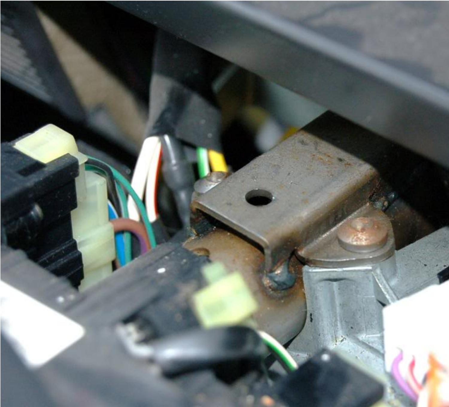
...when this is done you push **steering** ignition assembly down ...you can **see** steering lock pin...
