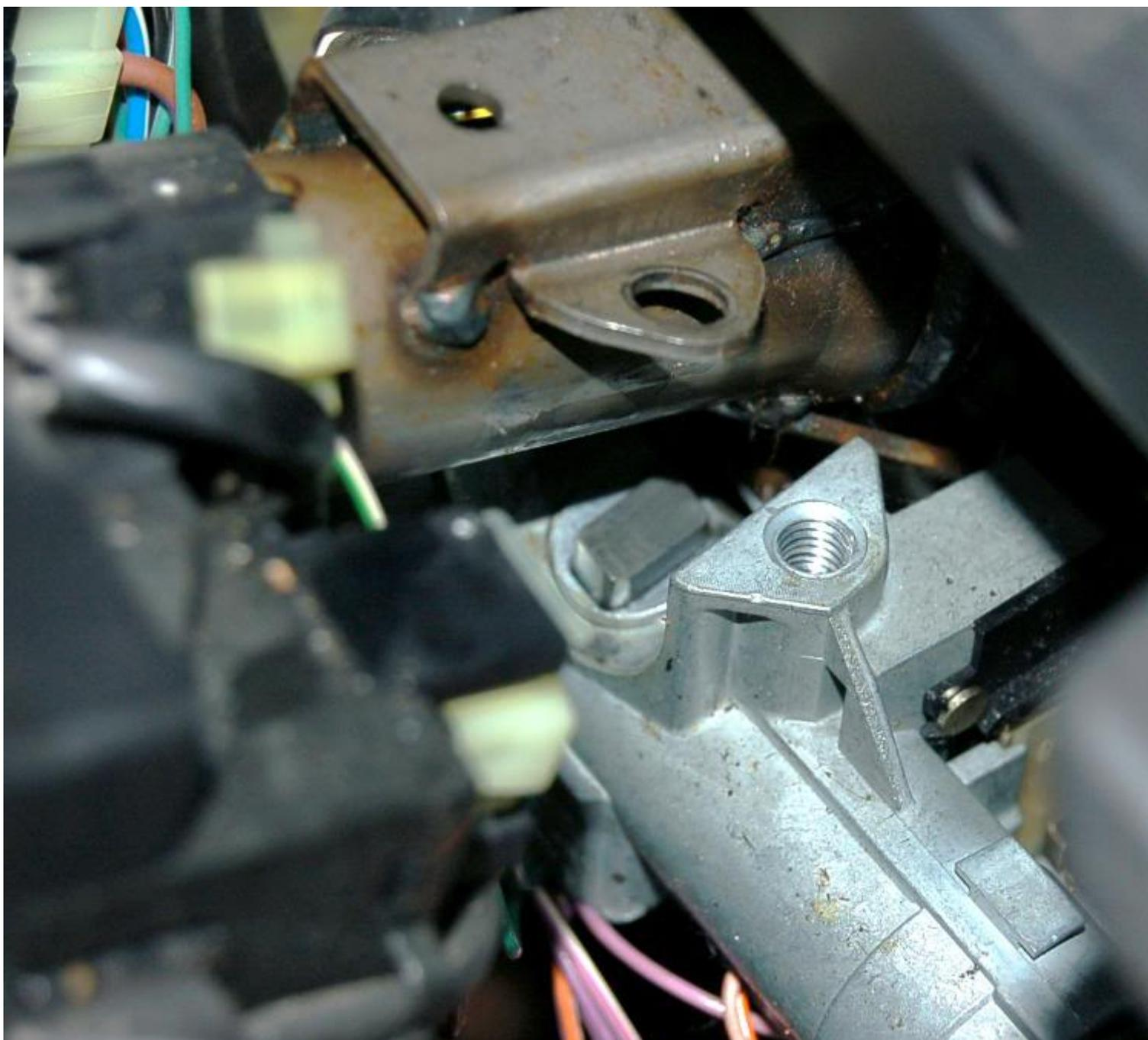
...on the left side you will see black **ignition** switch secured with two philips screws on each side...take those screws off...slide **ignition** switch out...at this point you can start your truck with flat screwdriver and drive it ...only thing you will not have is **steering** lock , which you don't need it for driving...so in case your steering repair take more time , your truck is in driving **condition**...
