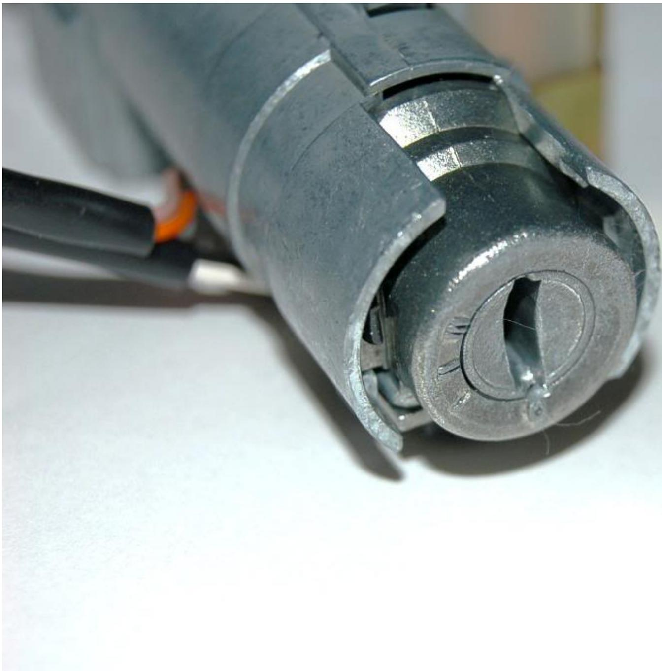
...on the side of the assembly you will see riveted safety pin...you will have to drill it out ...you can see how it look like removed...
