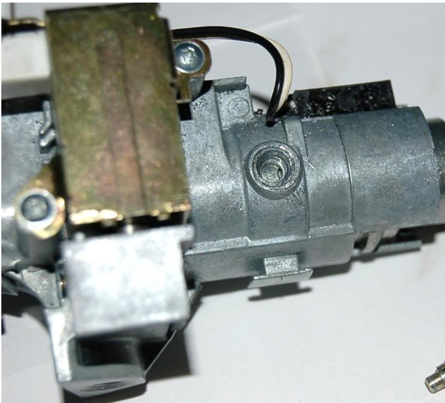
..now you can slide barrel out ... slowly ...first thing that will fall off is spring for the **ignition** buzzer ...don't lose it...that black thing is micro-switch for the ignition buzzer , you don't have to remove it...
