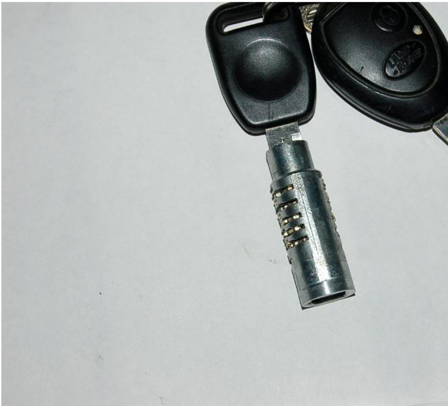
Installation is reverse of removal. I even used same [safety](#) pin to lock barrel back in to assembly. One who want to be really fancy , can retread it and use screw instead of the safety pin.
