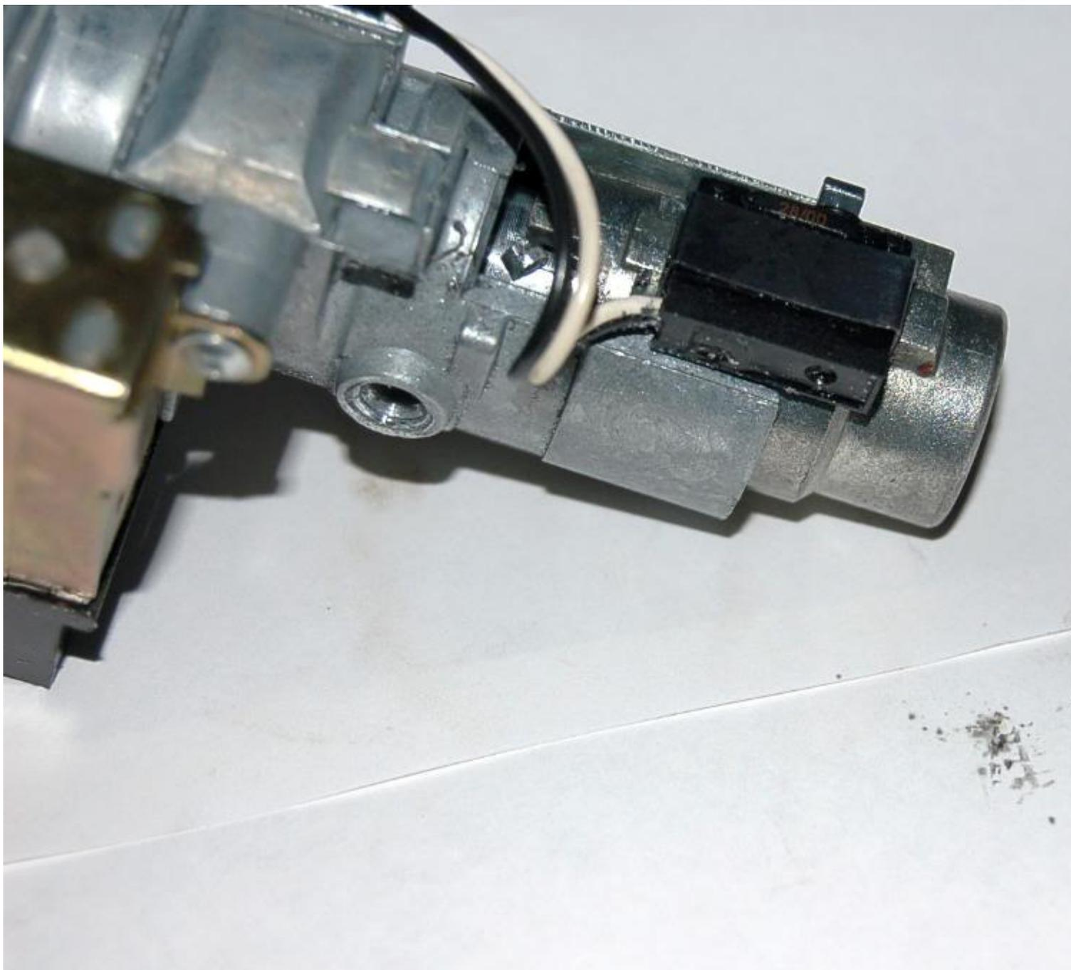
Once barrel is out , inside you will see spinner.Part that turns inside the barrel when you put key in to ignition.There are bras segments spring loaded , different for each lock combination.
