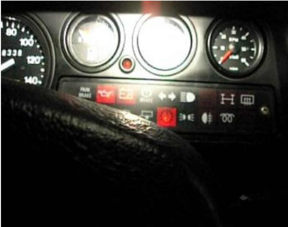
Photograph 4 Dash warning light. This light is unused and although not white on the instrument panel itself, the logo is there. It is between the trailer turning indicator light and the break warning light. It is a red warning light. You will need a small bulb.
