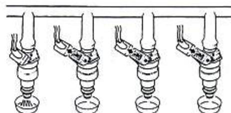
Ground Pin 11 and 16. This will cause the injectors to open. Place a large receptacle under the injector,
