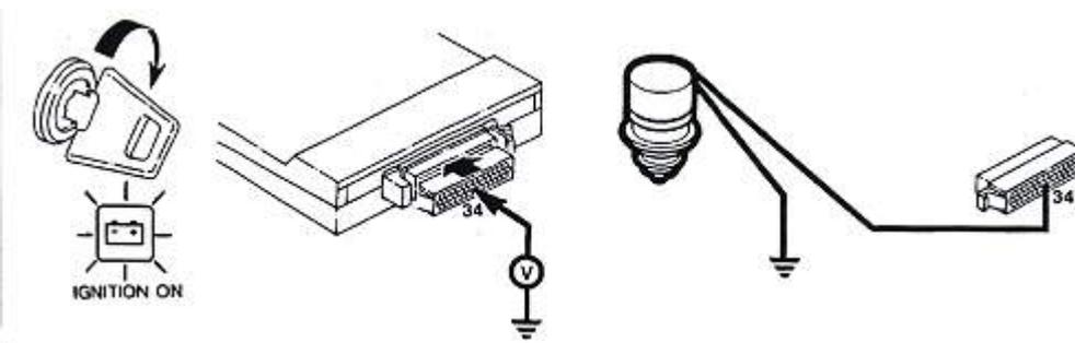
Connect voltmeter between Pin 34 and ground
