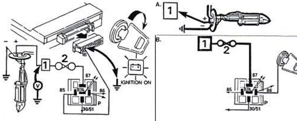
The pump is the in-tank model with connectors on the upper side of the tank- and inaccessible. However there is a connector not far away up the wiring harness where you can check voltage.
