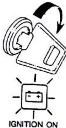
Voltmeter must show battery voltage. If 0Volt= see next step
