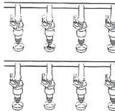
Injectors may leak. Take all the injectors out but don't disconnect them from the fuel rail. Put some sort of receptacle under them and switch on ignition. Any injector that gives off more than 2 drops a minute must be replaced.
