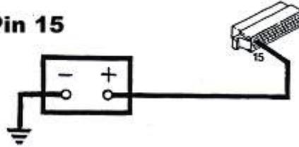
On the voltmeter the battery tension must show. (minimum 10V)
