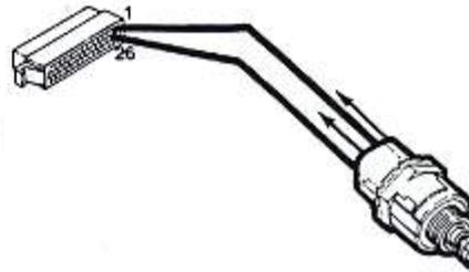
Connect ohmmeter between Pin 26 and 1.
