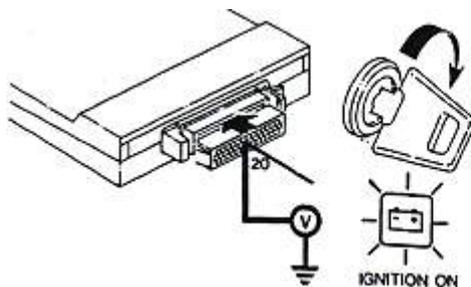
Connect voltmeter between Pin 20 and ground
