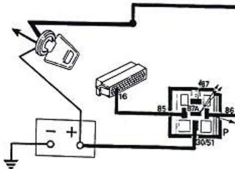
Pin 87 must show battery voltage if other conditions fulfilled.
