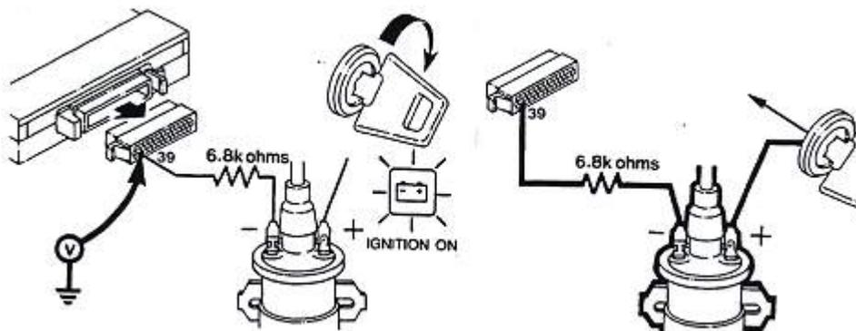
Check if Pin 39 has battery voltage on the voltmeter . Check resistance between coil and Pin 39 (6,8 KOhms)
