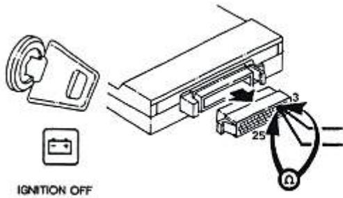
Connect ohmmeter between Pin 25 and 3.
