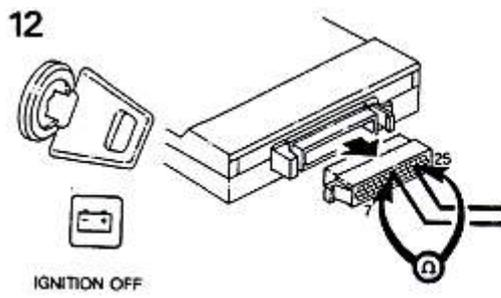
Connect ohmmeter between Pin 25 and 7.
