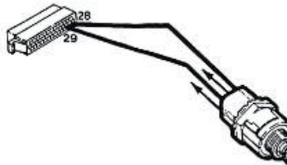
Connect ohmmeter between Pin 28 and 29.
