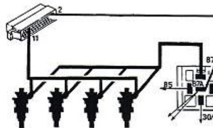
Connect ohmmeter between Pin 2 and 11. Reading of 4-5 ohms is OK.
