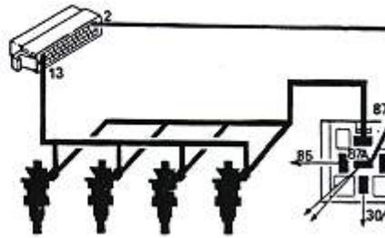
Connect ohmmeter between Pin 2 and 13. Reading of 4-5 ohms is OK.
