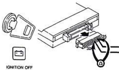
Connect ohmmeters between Pin 25 and 32.
