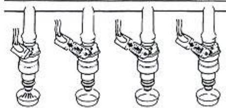
Ground Pin 13 and 16. This will cause the injectors to open. Place a large receptacle under the injector, maybe a bottle or so. A correct injector will flow **167 cm<sup>3</sup> per minute!**
