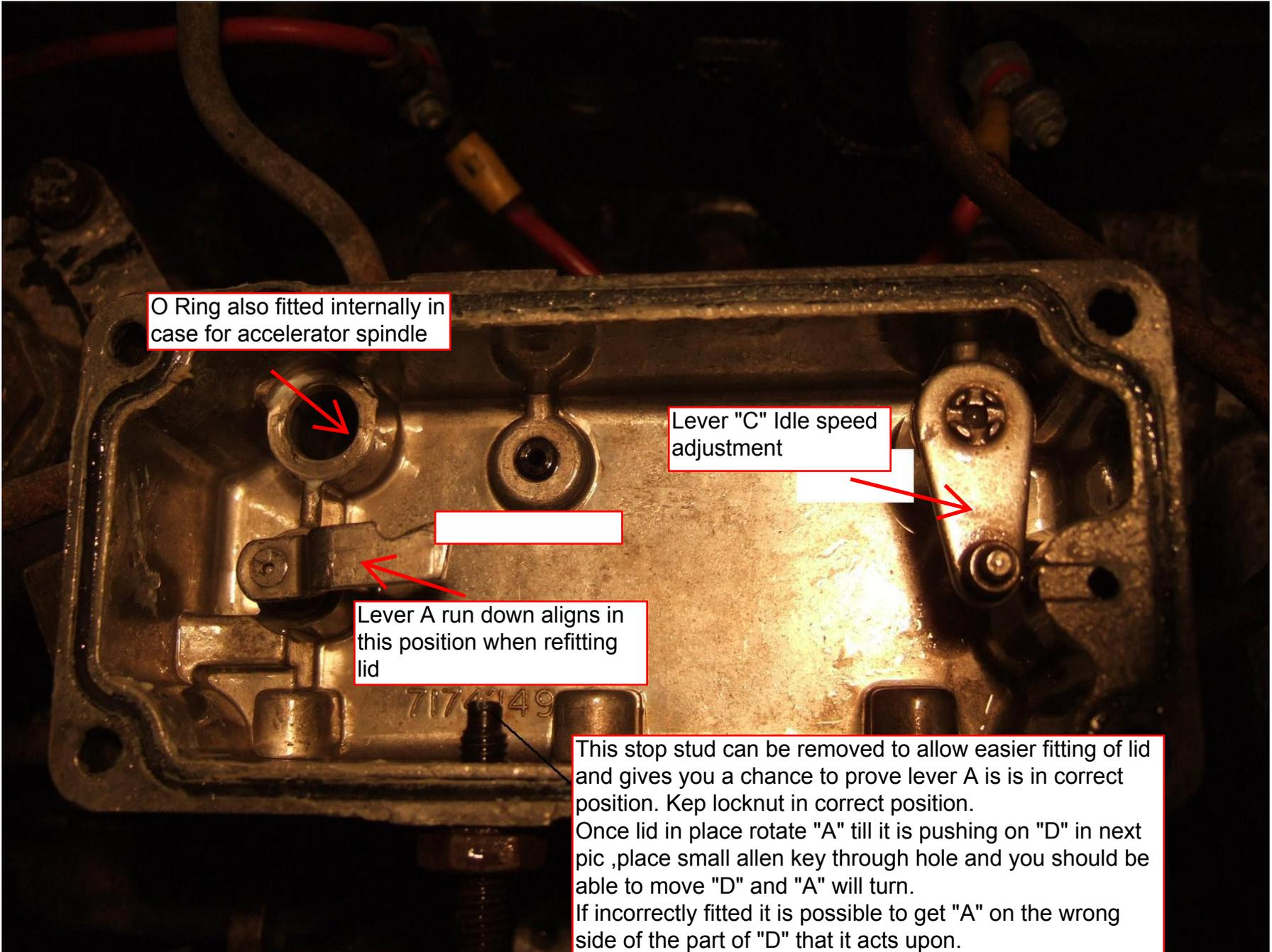
O Ring also fitted internally in case for accelerator spindle
