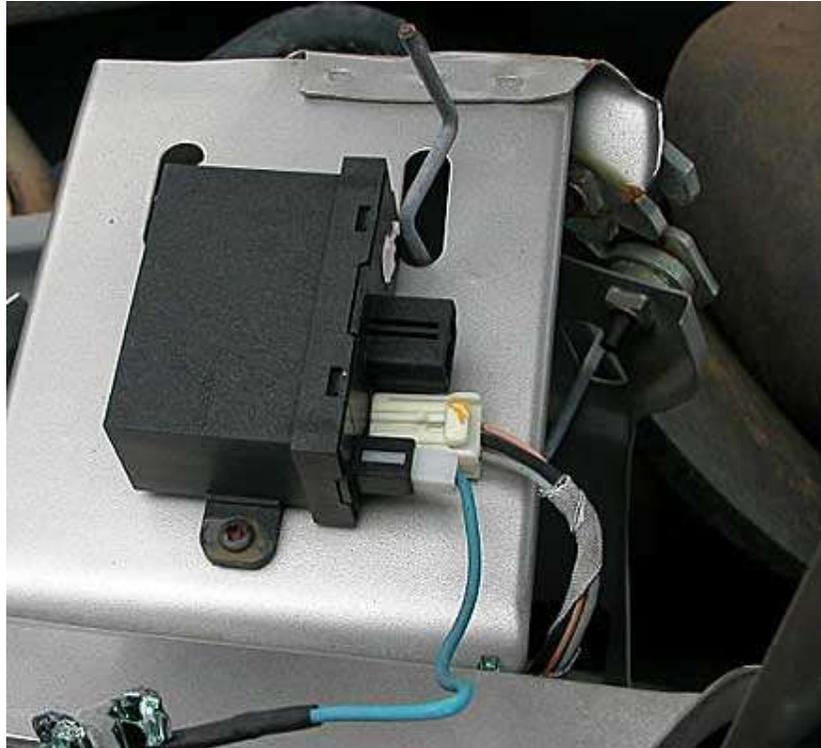
appears to be a magnetic field generated by an LPG pump which seems to interrupt not only the handset signaling the locks but also the handset talking to the BeCM when inserted into the ignition switch, preventing the car from starting. (He managed to get around this problem by manually locking the vehicle with the key in the door lock when he gets out at the station and then everything works fine when he gets back in).
