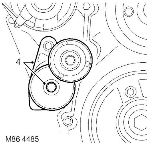
4. Remove bolt (LH thread) and remove auxiliary drive belt tensioner.
