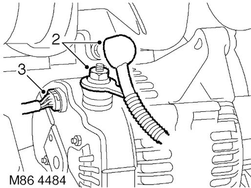
2. Release cover and remove nut securing lead to alternator.
