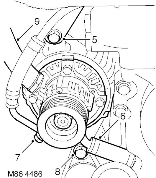
5. Remove bolt securing support stay to alternator.
