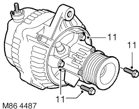
11. Remove 4 bolts, and remove vacuum pump from alternator.
