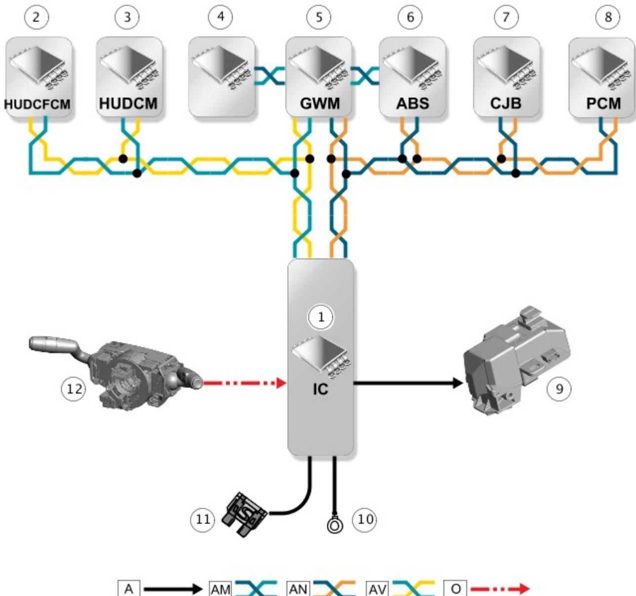
A = Hardwired; AM = High Speed (HS) Controller Area Network (CAN) Chassis systems bus; AN = HS CAN Powertrain systems bus; AV = HS CAN Comfort systems bus.
